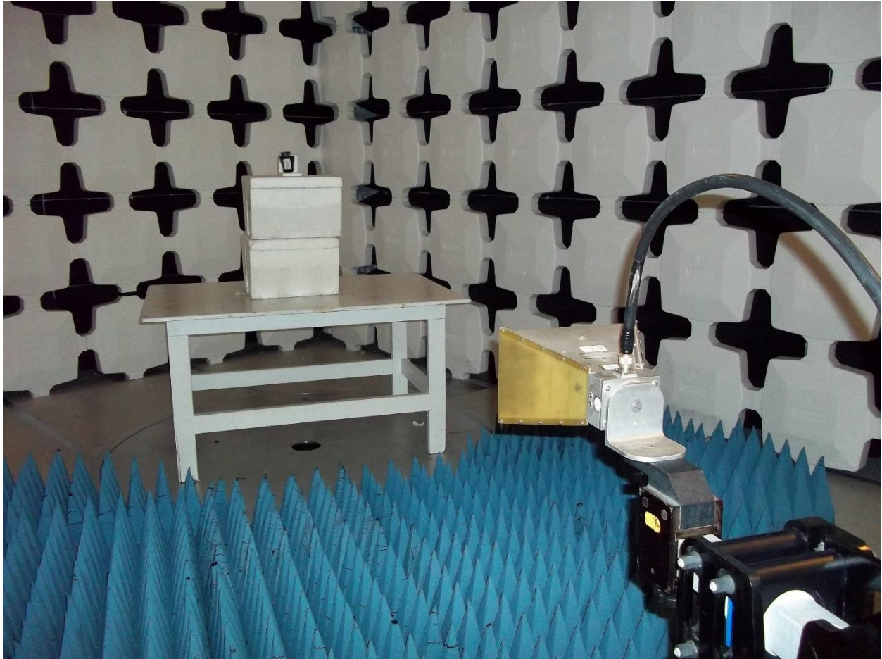
Figure 4. Radiated Emissions Test Configuration (> 1 GHz)
