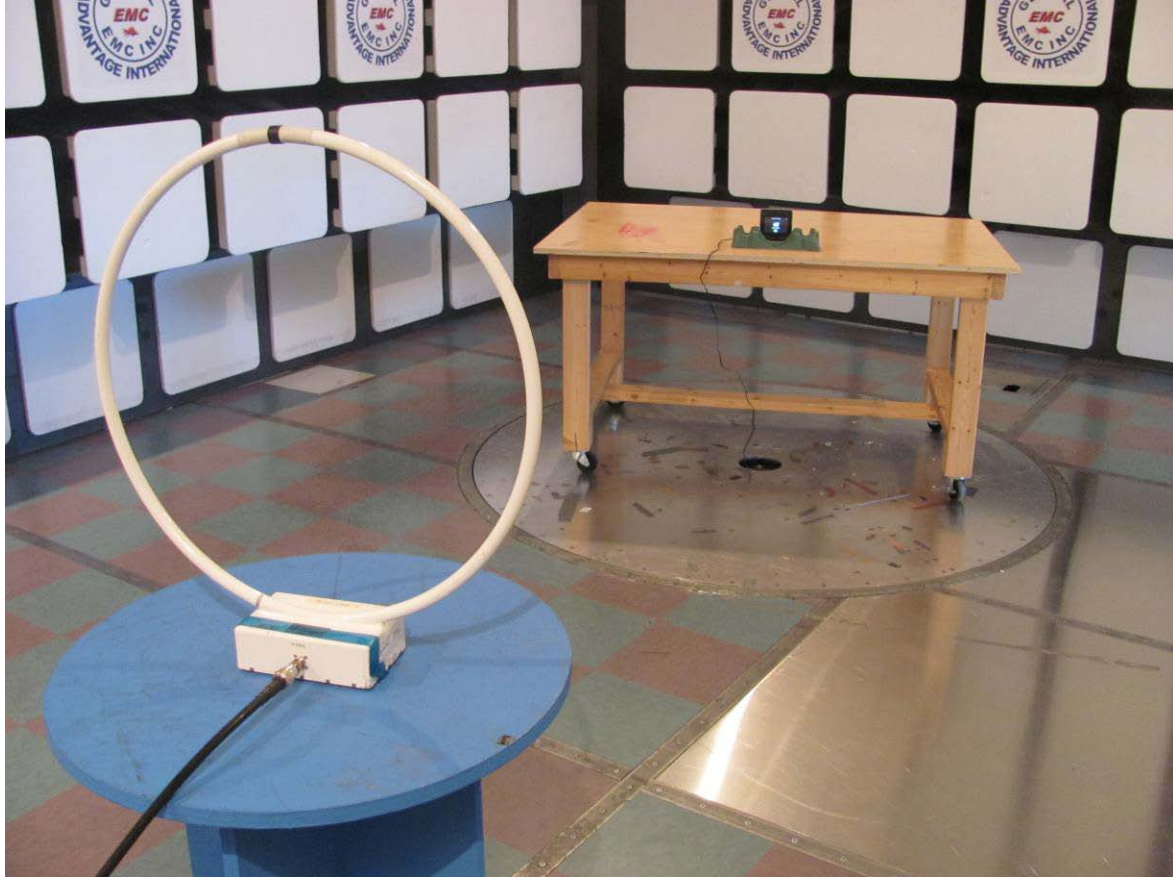
Figure 1: Radiated emission setup – photo 1
