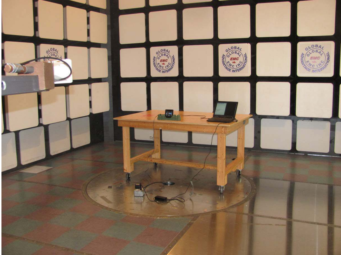
Figure 3: Radiated emission setup – photo 3
