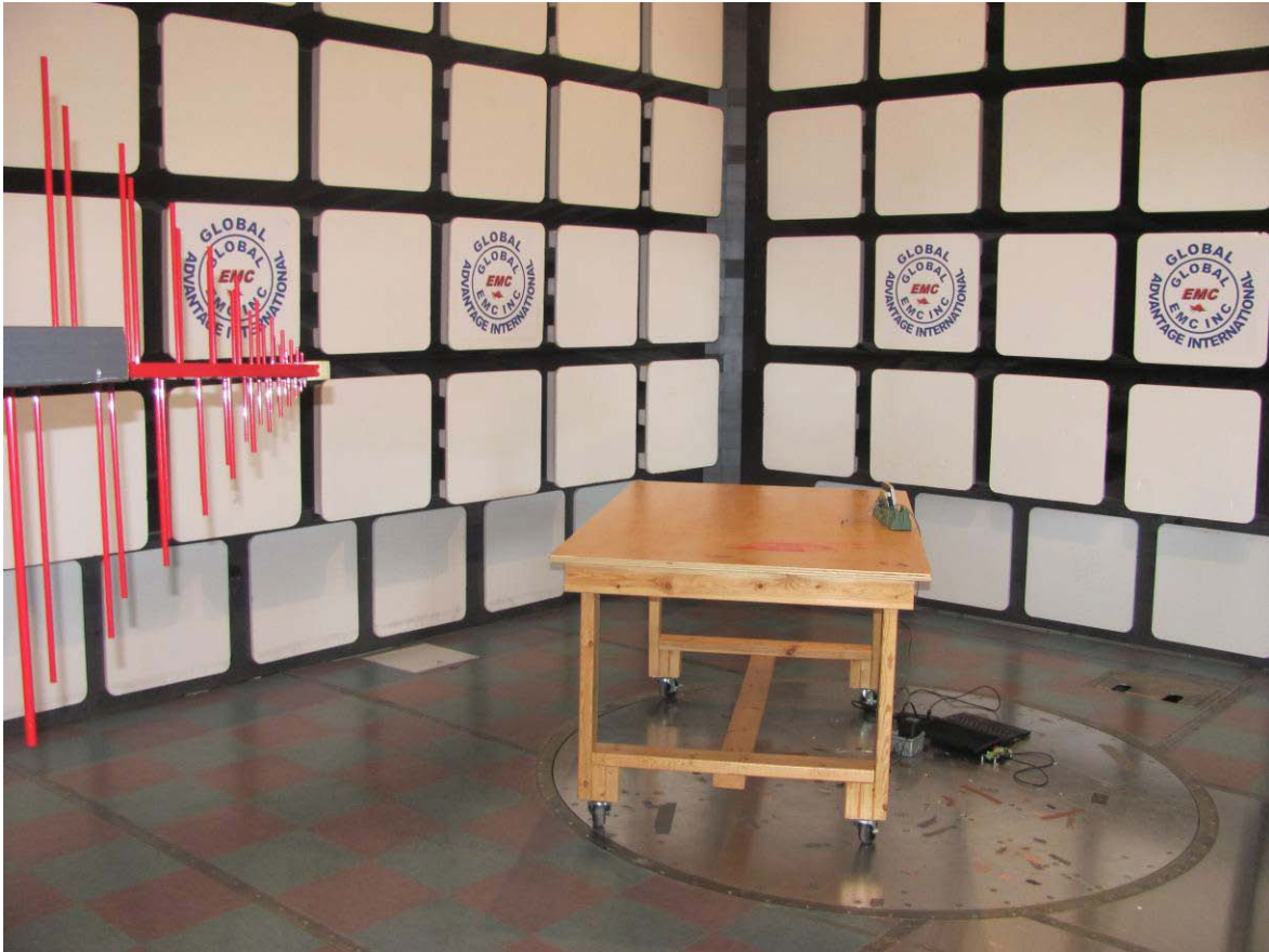
Figure 5: Radiated emission setup – photo 2
