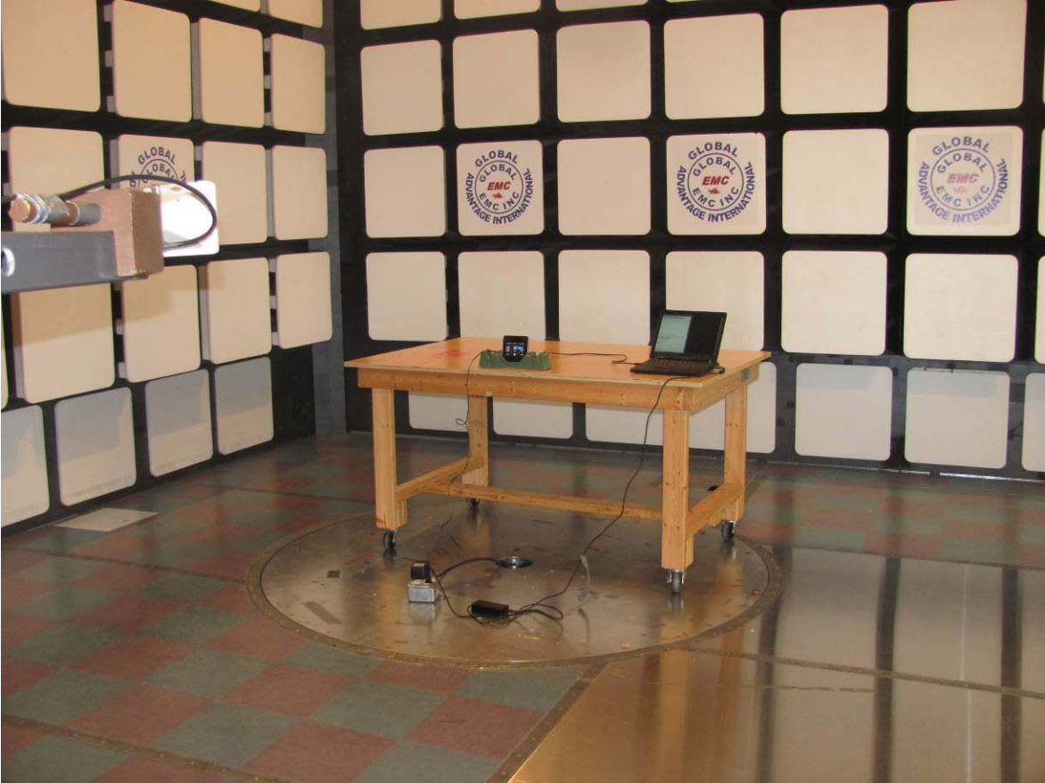
Figure 6: Radiated emission setup – photo 3
