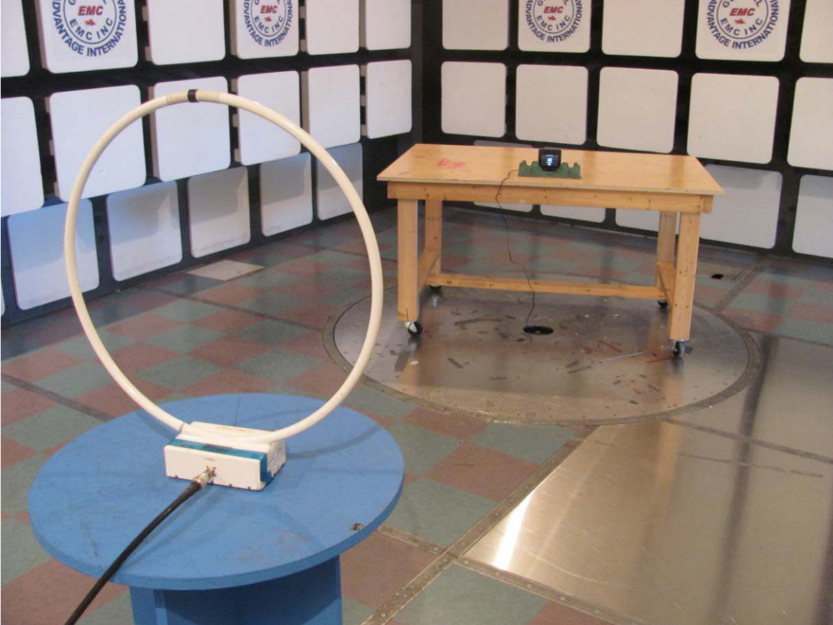
Figure 4: Radiated emission setup – photo 1
