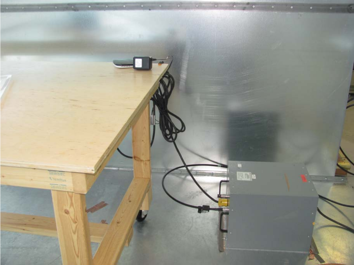
Illustration 7: Power line conducted emission setup – photo 1
