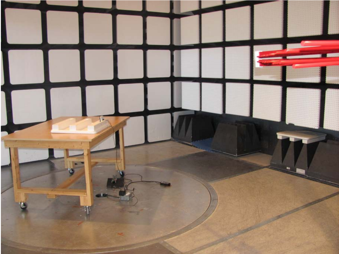
Illustration 4: Radiated emission setup - photo 2
