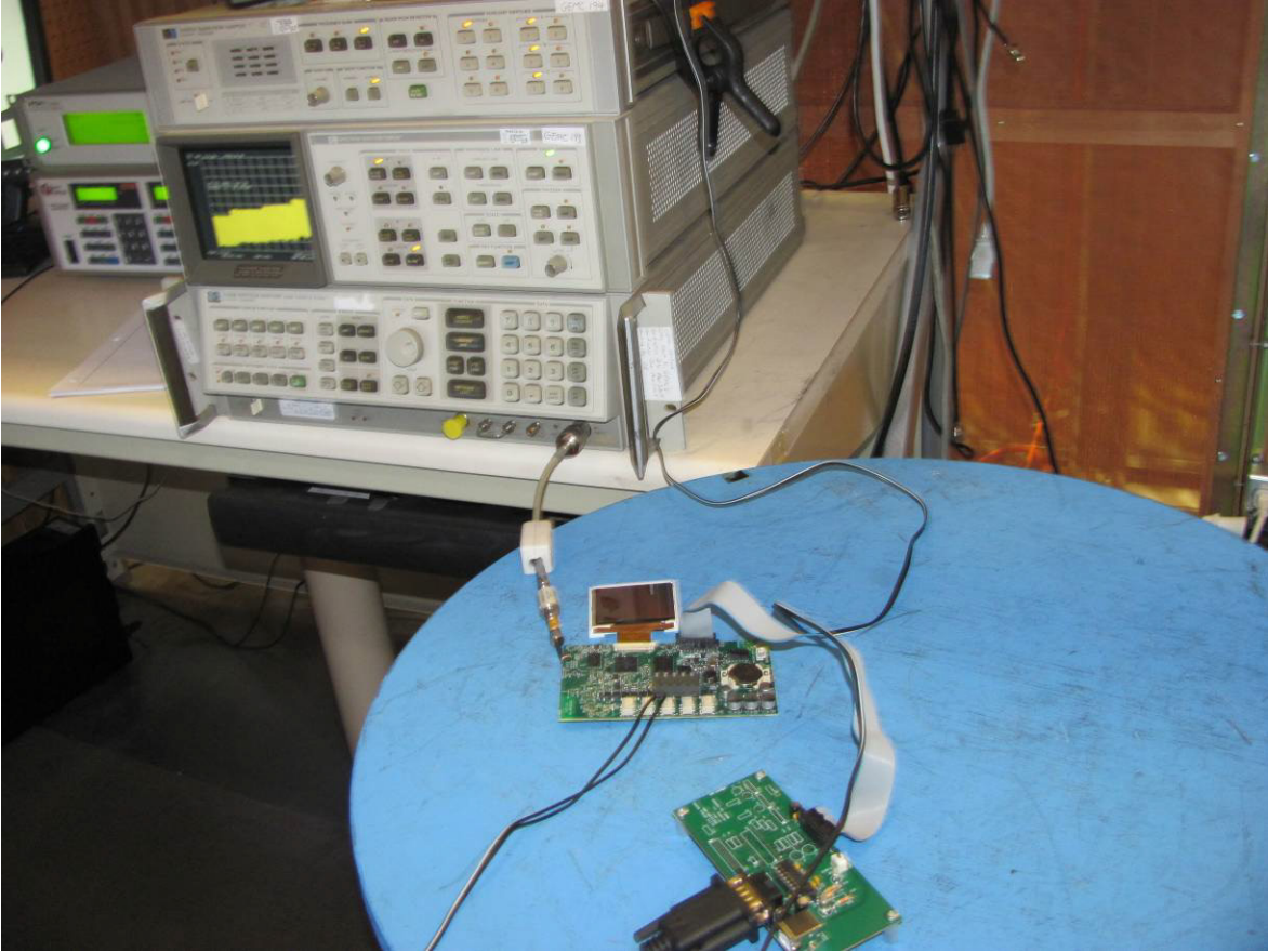
Figure 7: Antenna port conducted emission setup – photo
