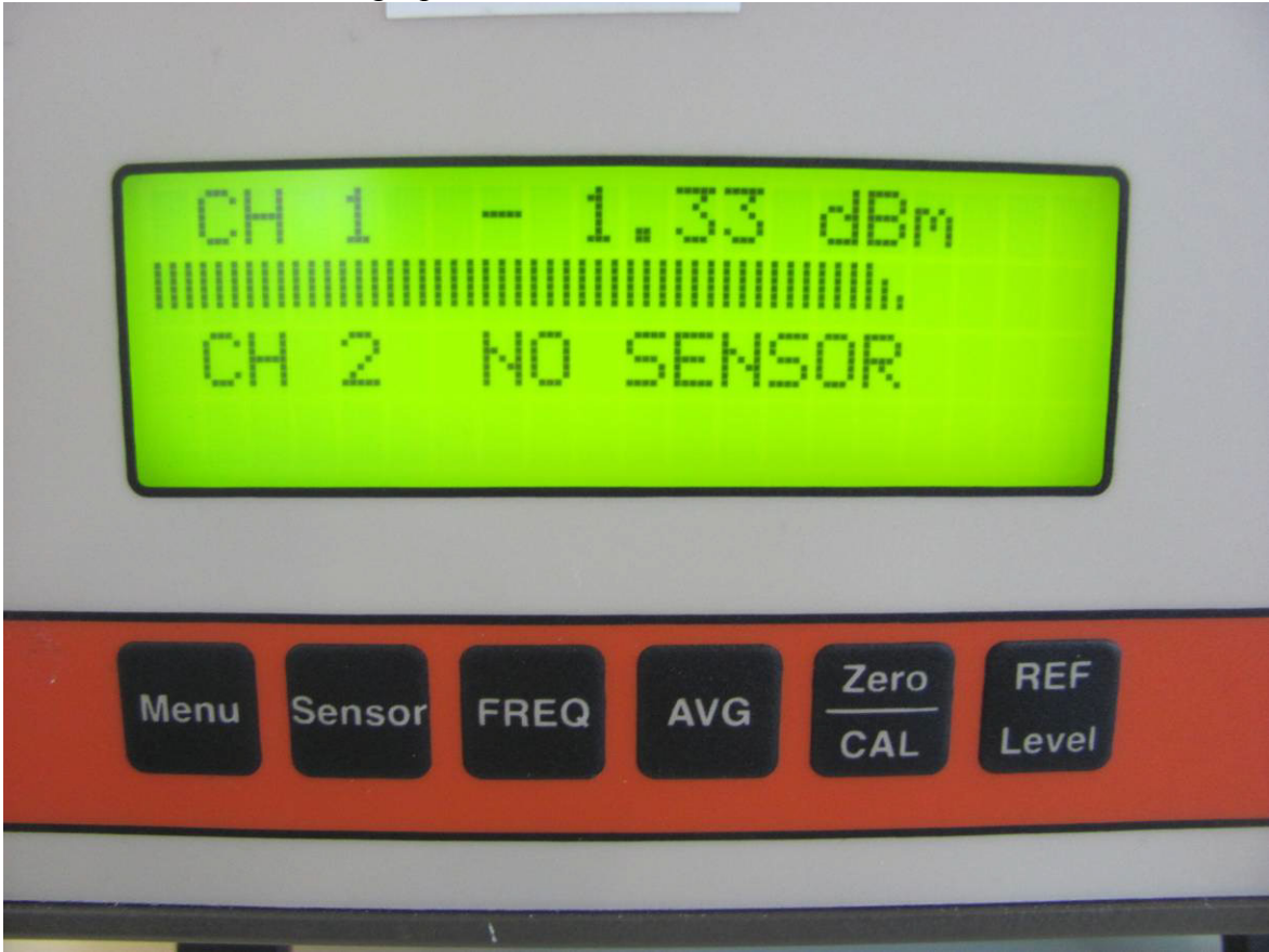
Figure 1: Power reading of B Protocol, Mid channel - photo
