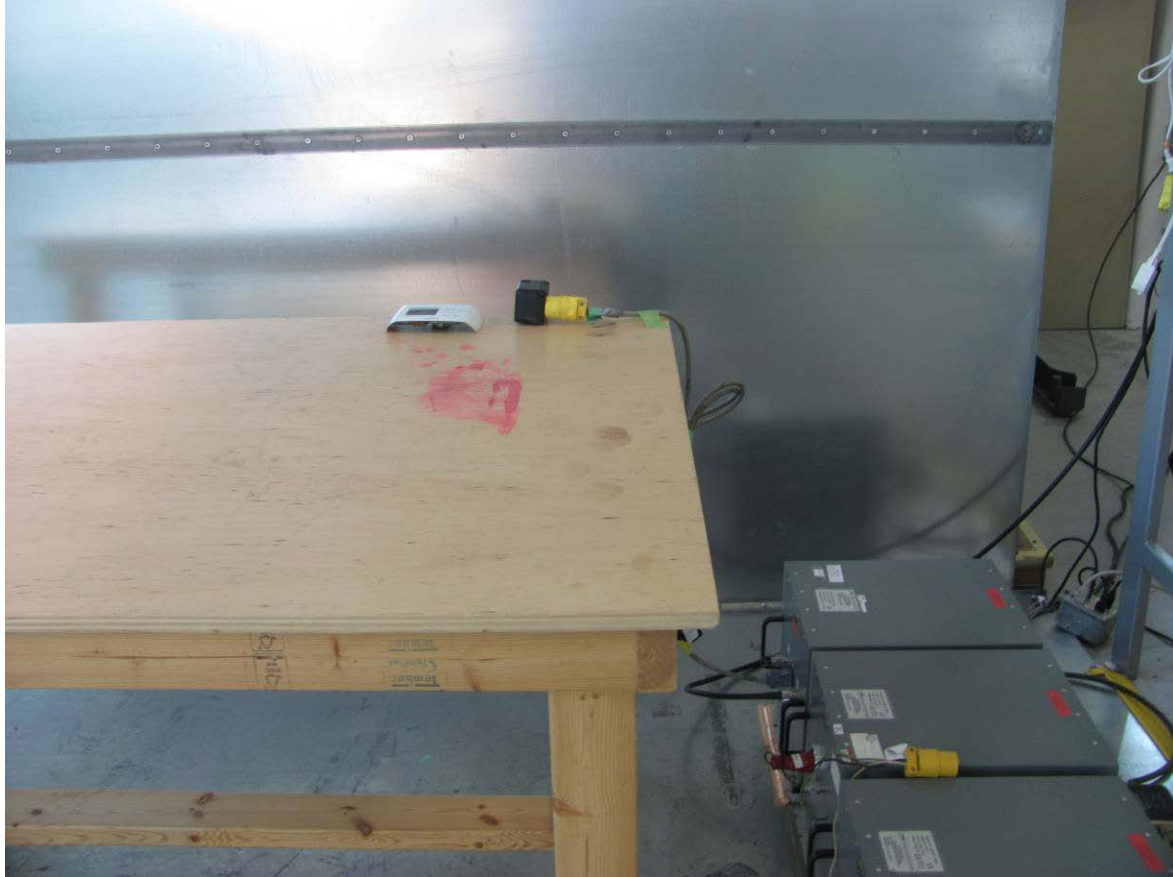
Figure 7: Power line conducted emission setup – photo 1
