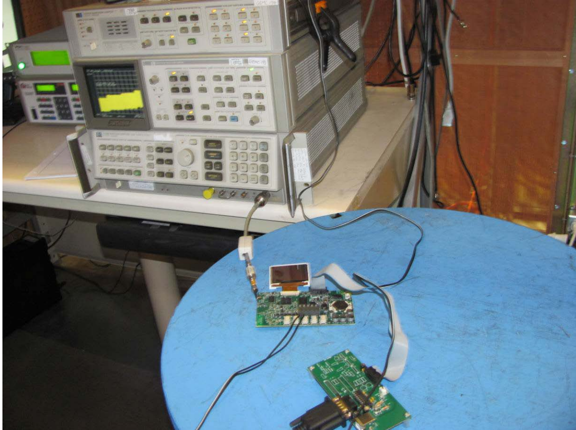
Figure 5: Antenna port conducted emission setup – photo
