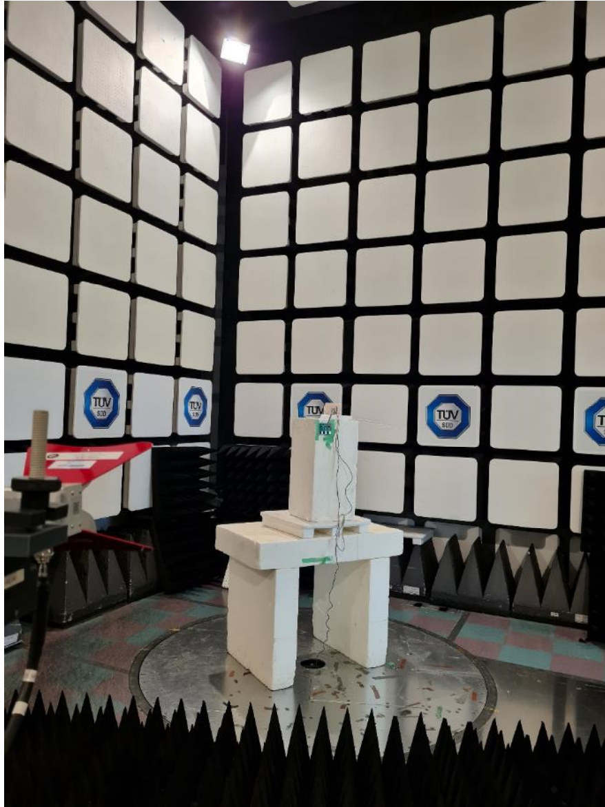
Figure 4 – Radiated Emissions Setup > 1GHz
