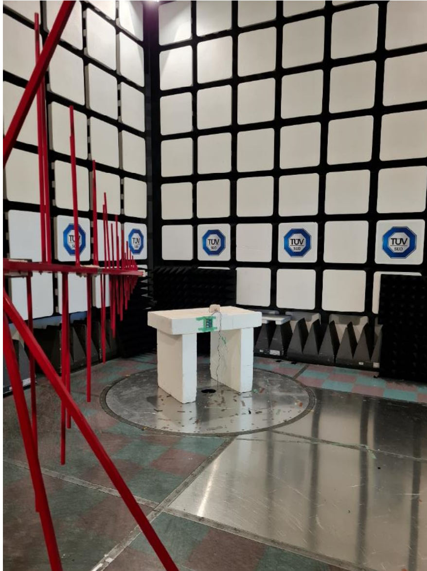
Figure 3 – Radiated Emissions Setup 30MHz – 1GHz
