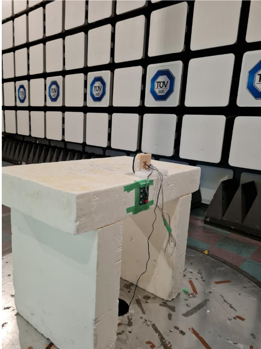
Figure 1 – Radiated Emissions Setup
