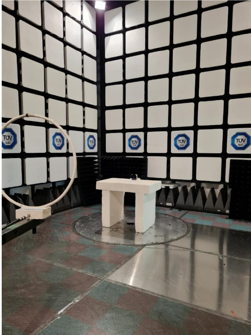
Figure 2 – Radiated Emissions Setup 9kHz – 30MHz
