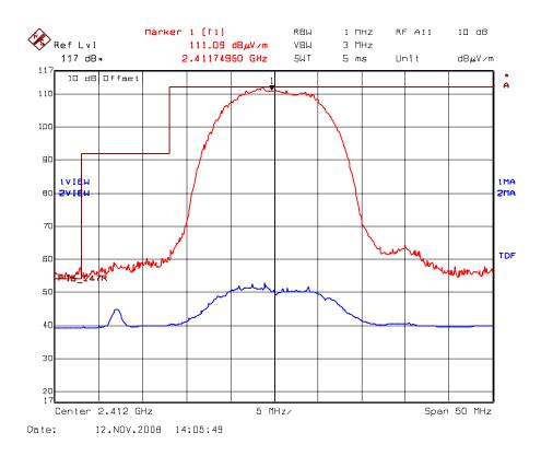
Trace 1: RBW= 1 MHz, VBW= 3 MHz Trace 2: RBW= 1 MHz, VBW= 10Hz
