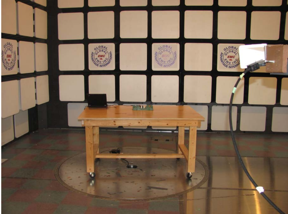
Illustration 2: Radiated emission setup - photo 2
