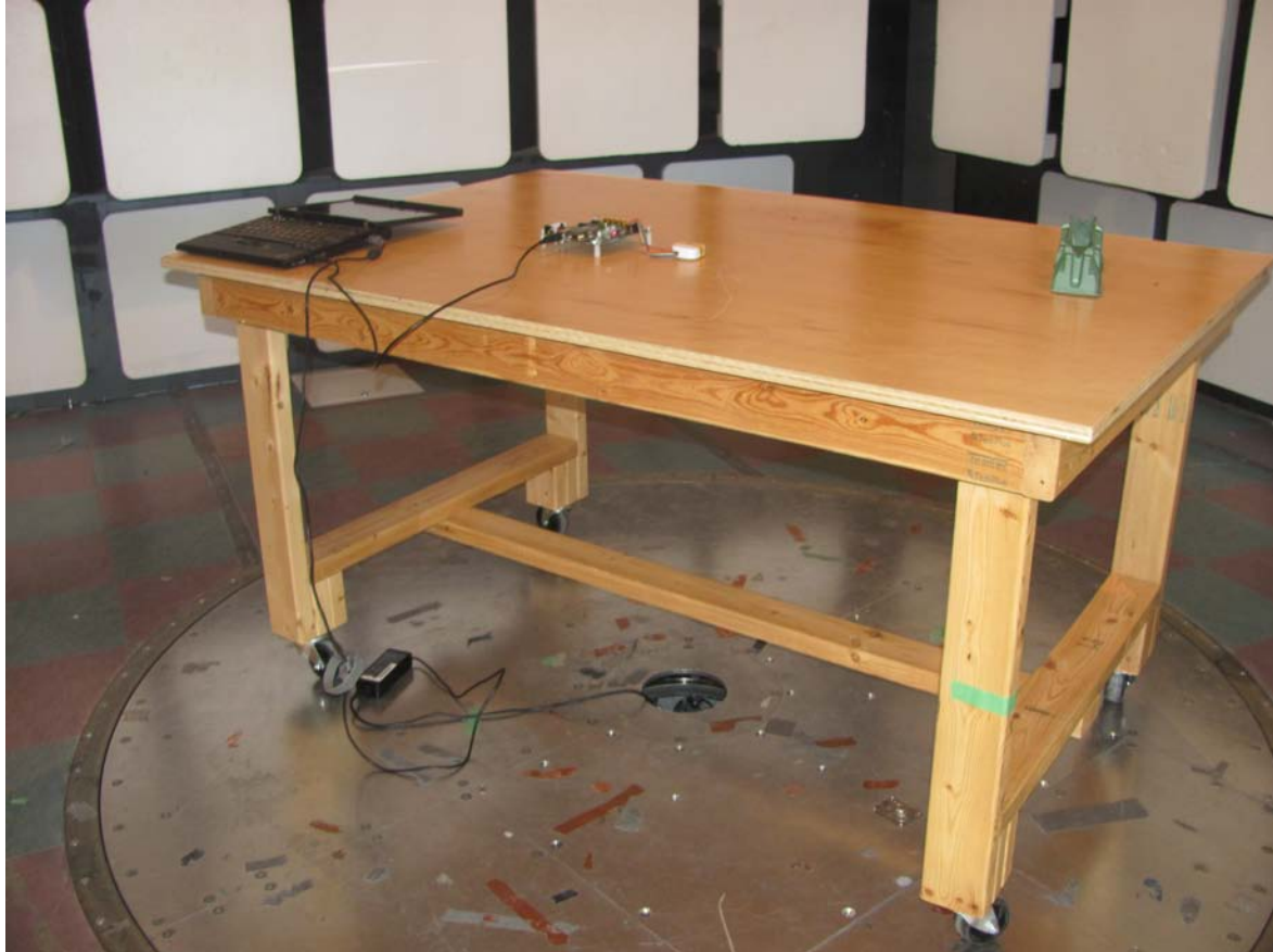
Illustration 1: Radiated emission setup – photo 1
