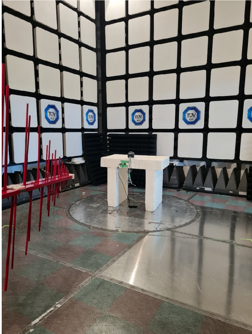
Figure 1 – Radiated Emissions Setup 30MHz – 1GHz
