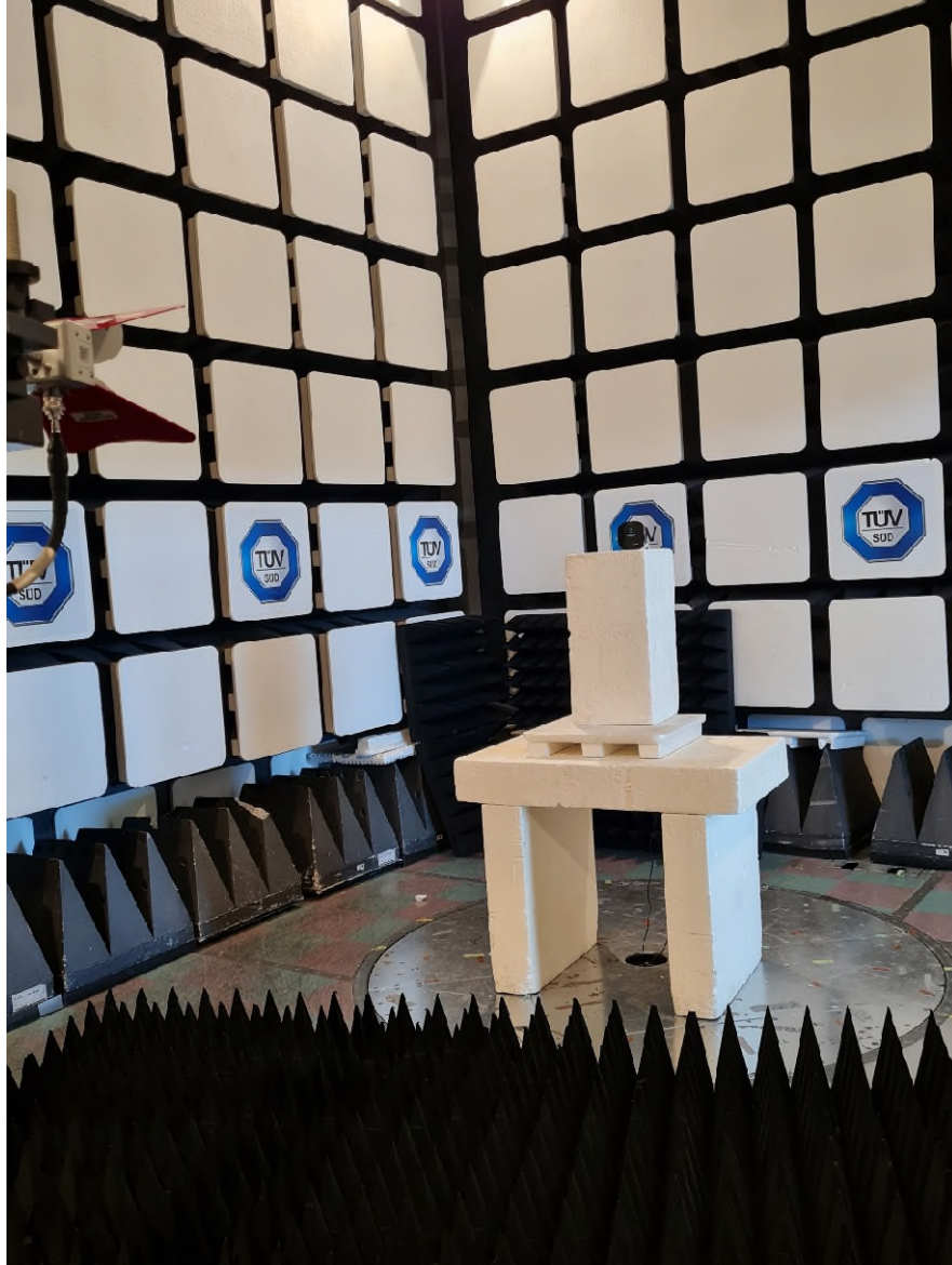
Figure 2 – Radiated Emissions Setup > 1GHz
