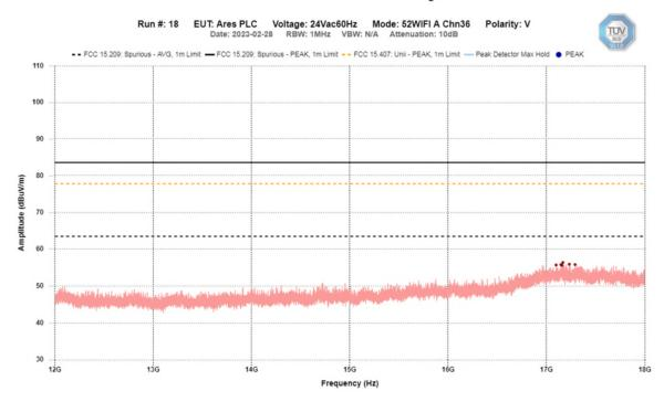
Plot was taken at a 1 meter distance. All emissions were noise floor of measurement instrument. No emissions were found in this frequency range.
