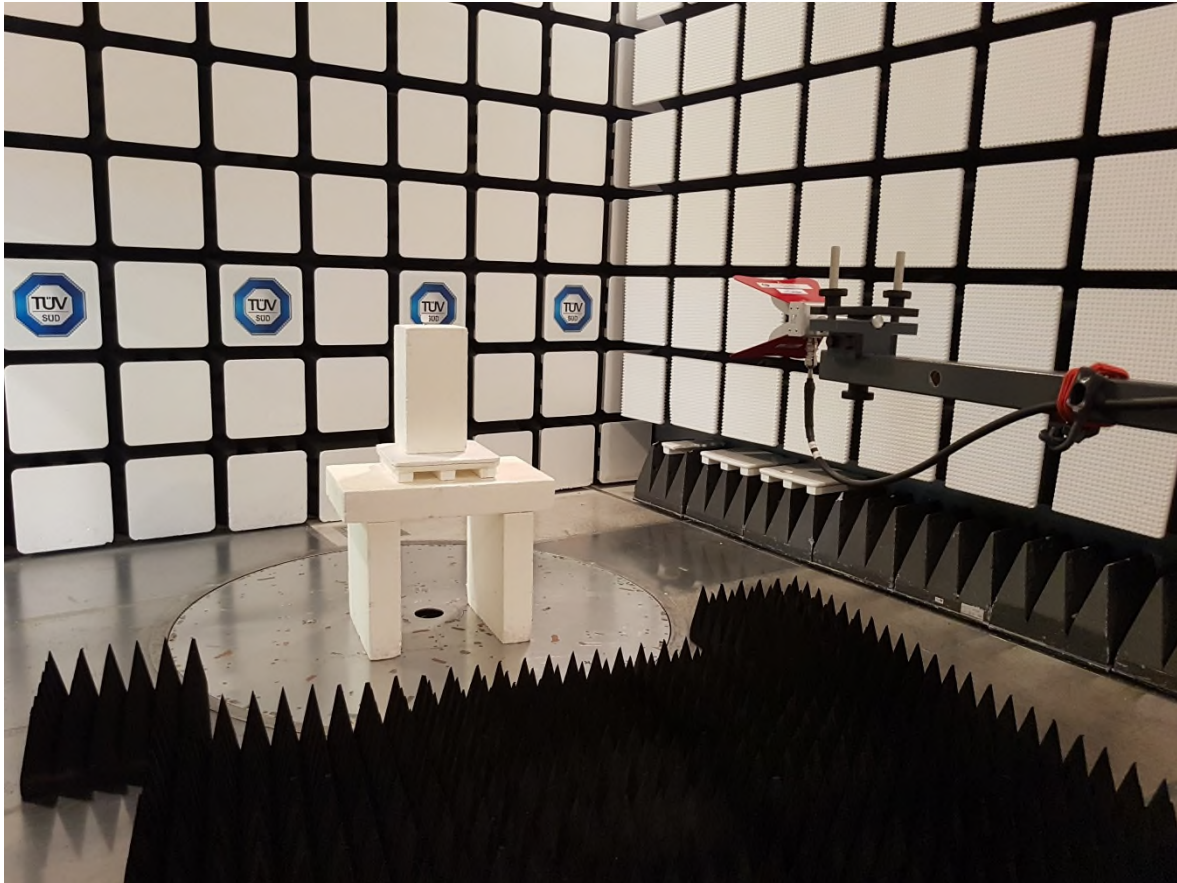
Figure 5 – Radiated Emissions Setup 1GHz – 10GHz
