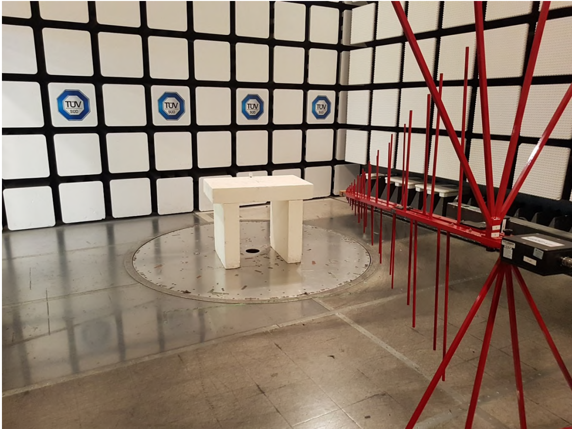
Figure 4 – Radiated Emissions Setup 30MHz – 1GHz
