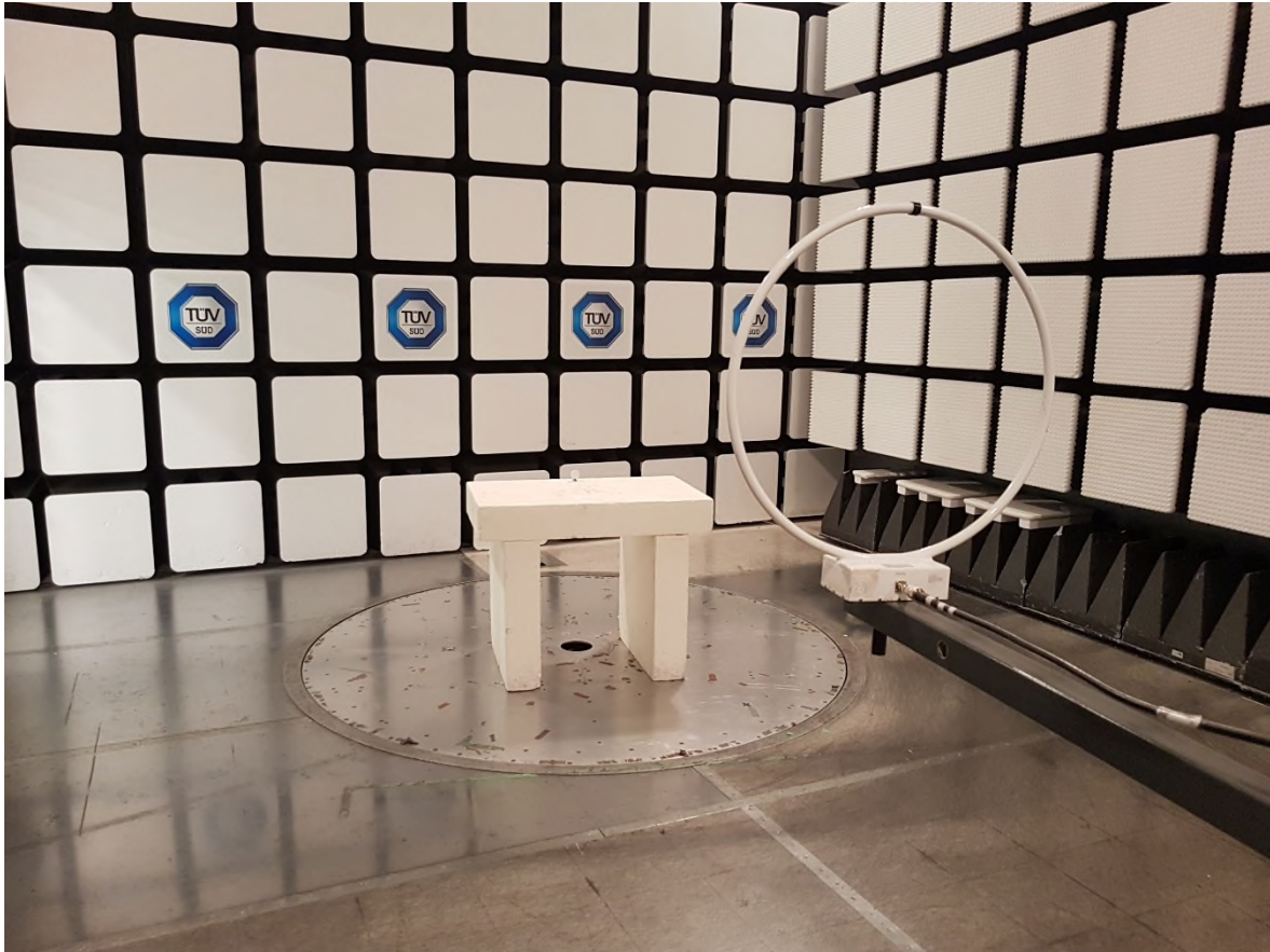
Figure 3 – Radiated Emissions Setup 9kHz – 30MHz
