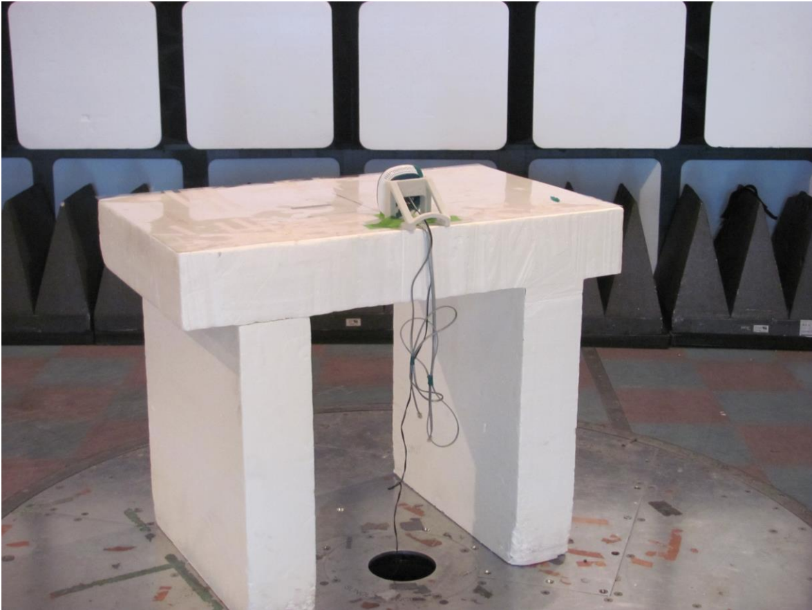
Figure 1 – Radiated Emissions Setup – Photo 1
