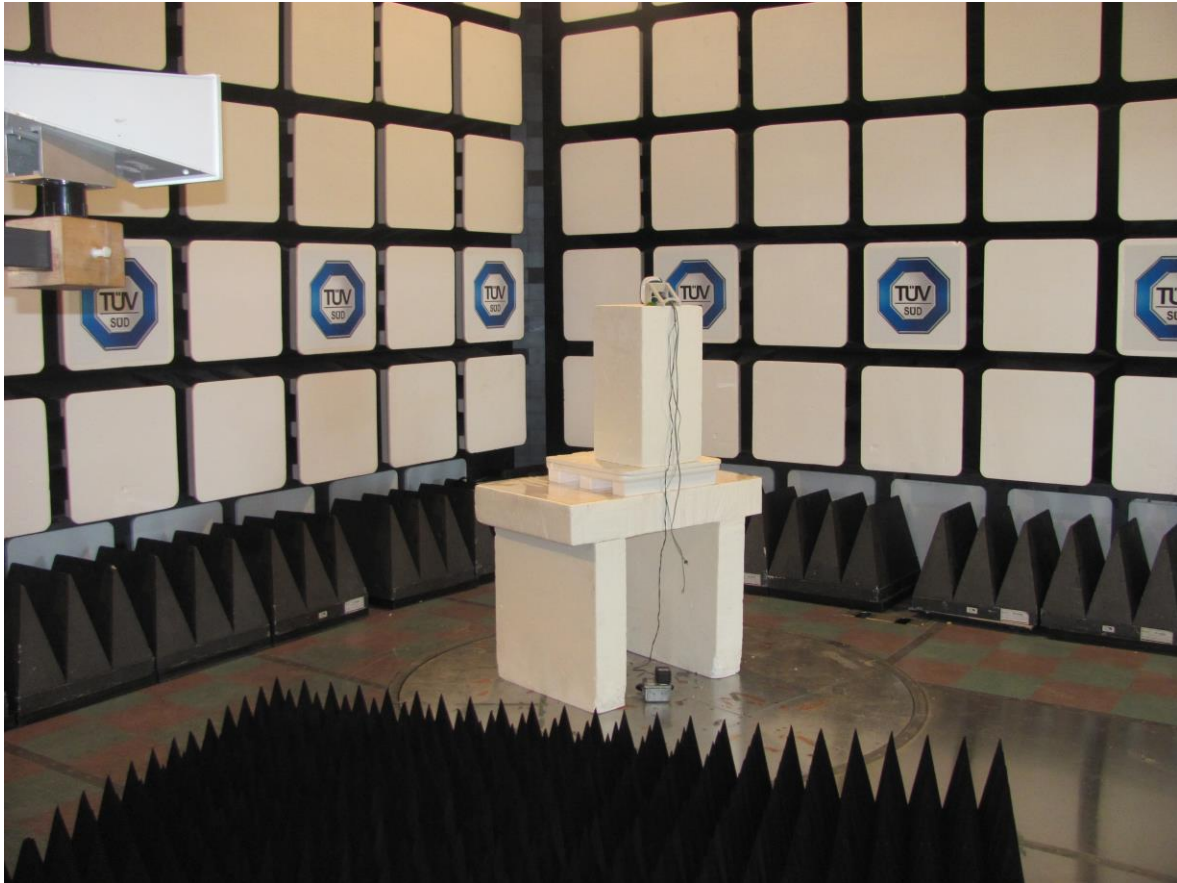
Figure 4 – Radiated Emissions Setup – Photo 4
