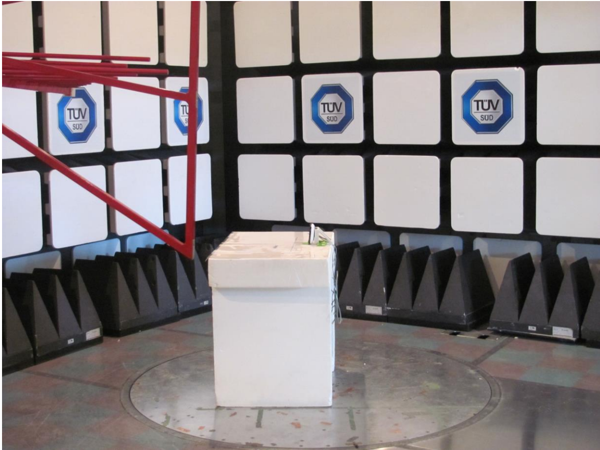
Figure 3 – Radiated Emissions Setup – Photo 3
