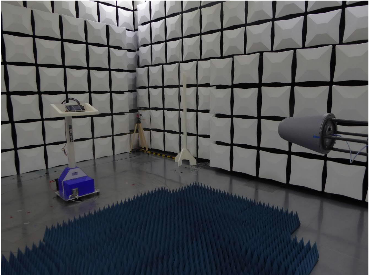
Test setup – radiated test in anechoic chamber (M276)
