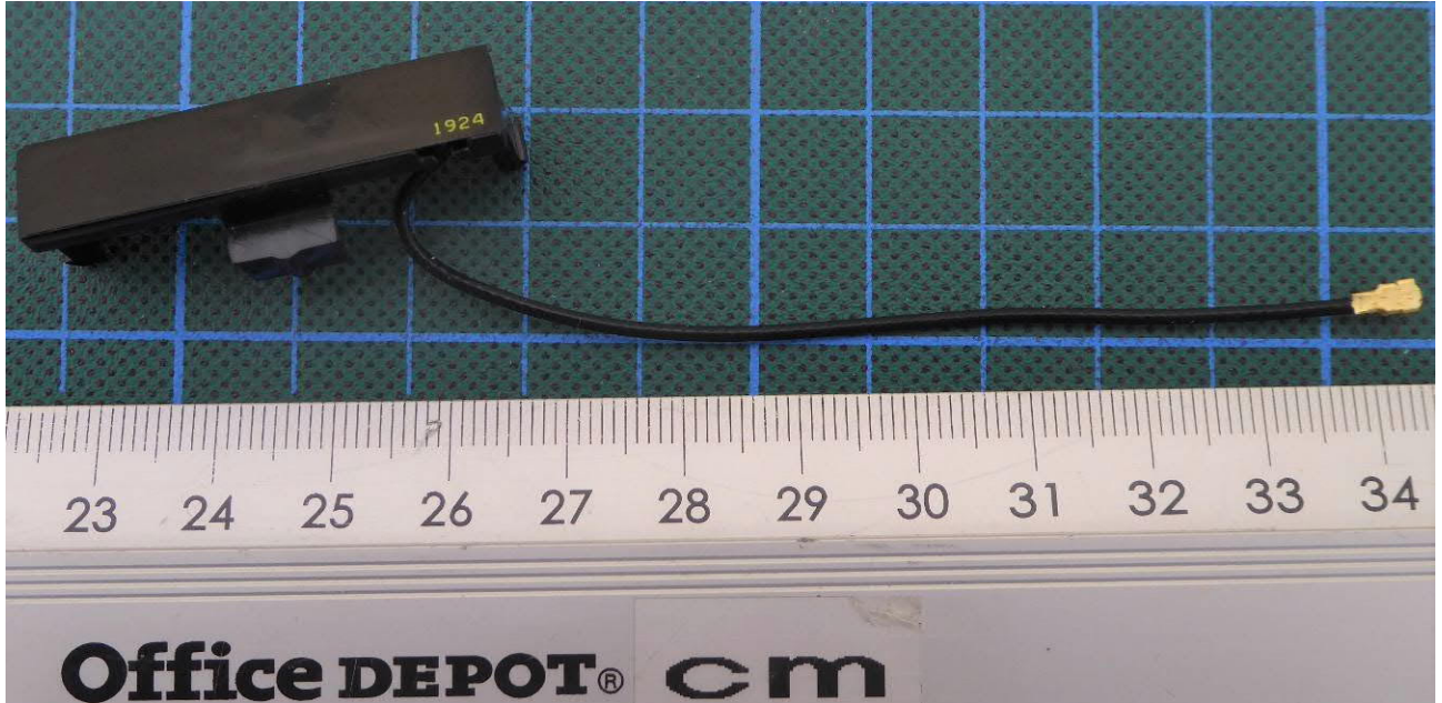
Antenna – top view
