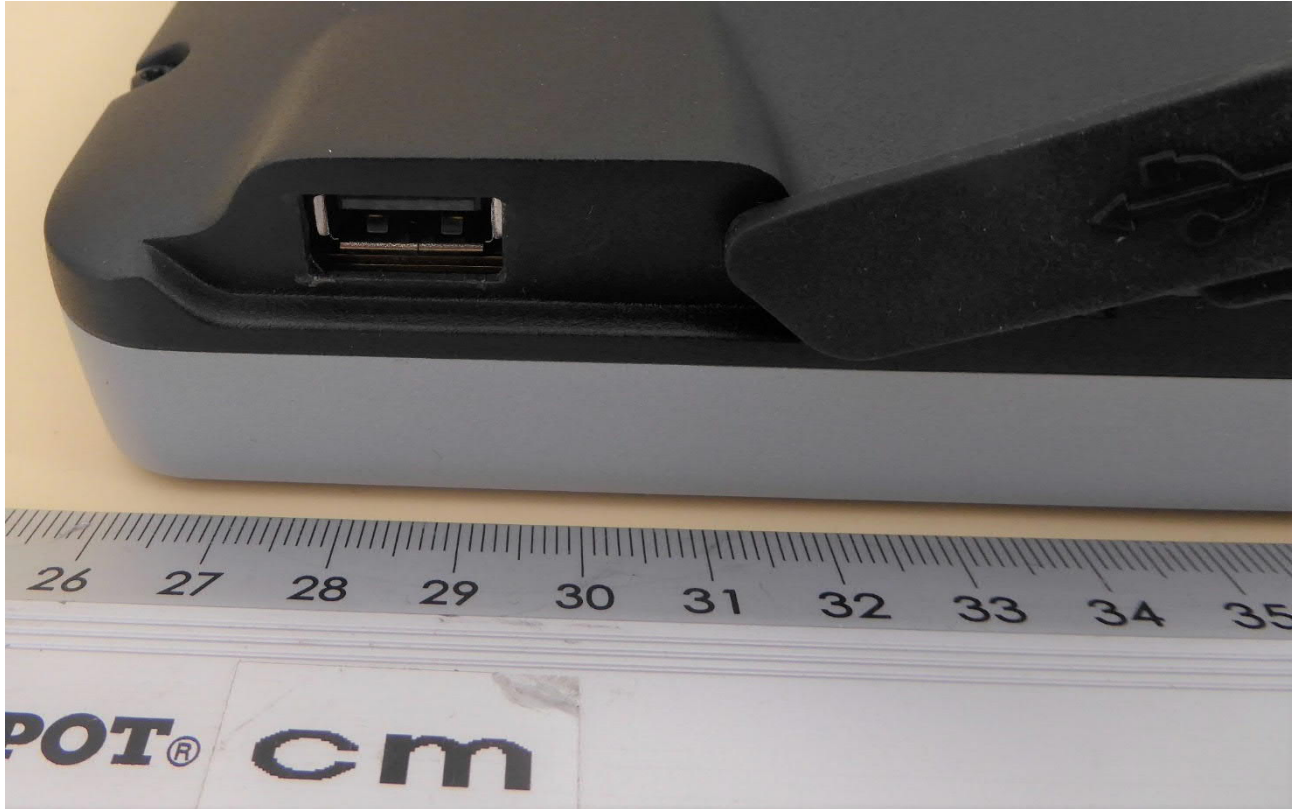
EUT – USB interface cover opened
