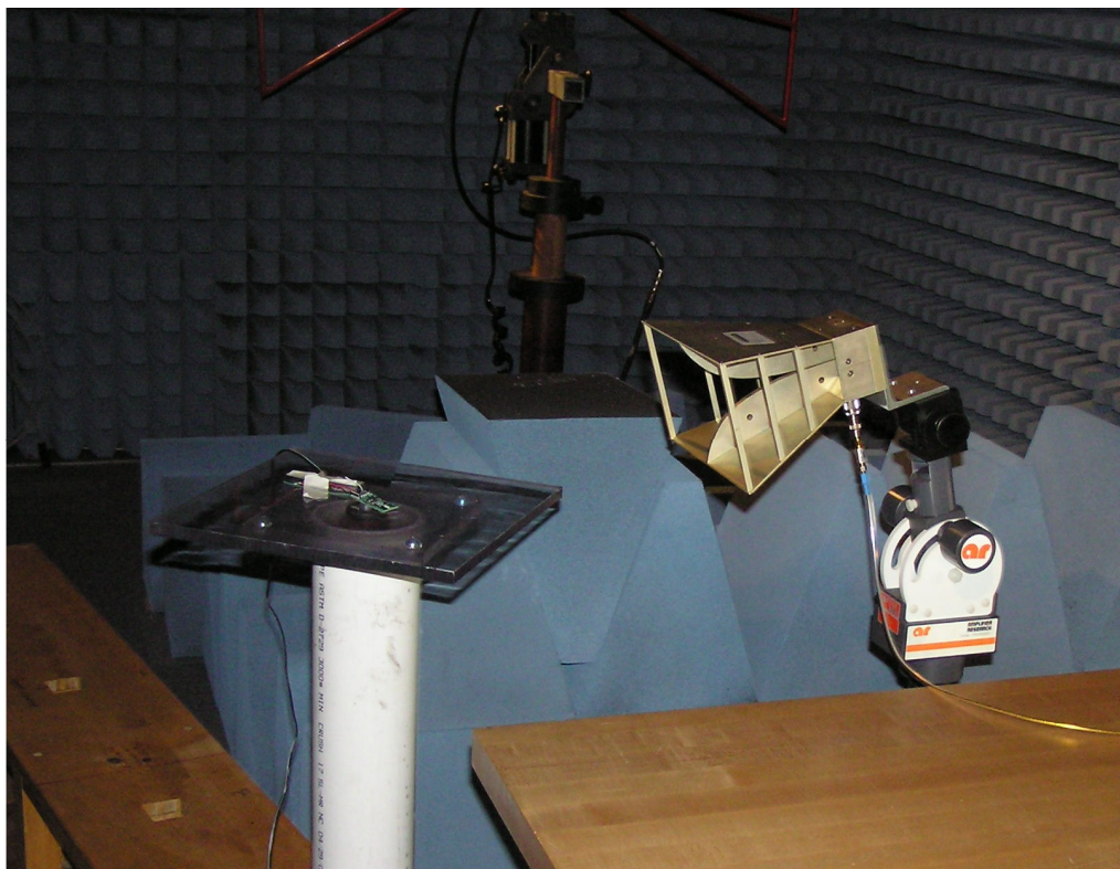
Figure 11 Setup Radiated Harmonic Emissions Measurements
