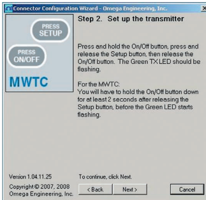
Figure 4-6 Setup The Transmitter Screen
