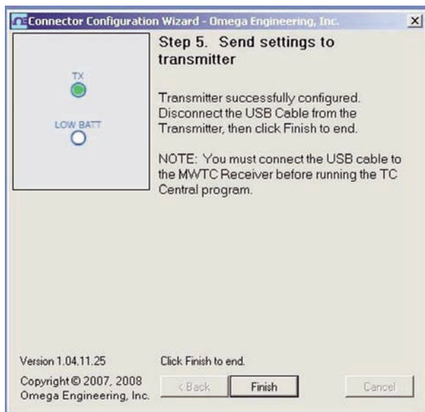
Figure 4-10 Send Settings To Transmitter Screen
