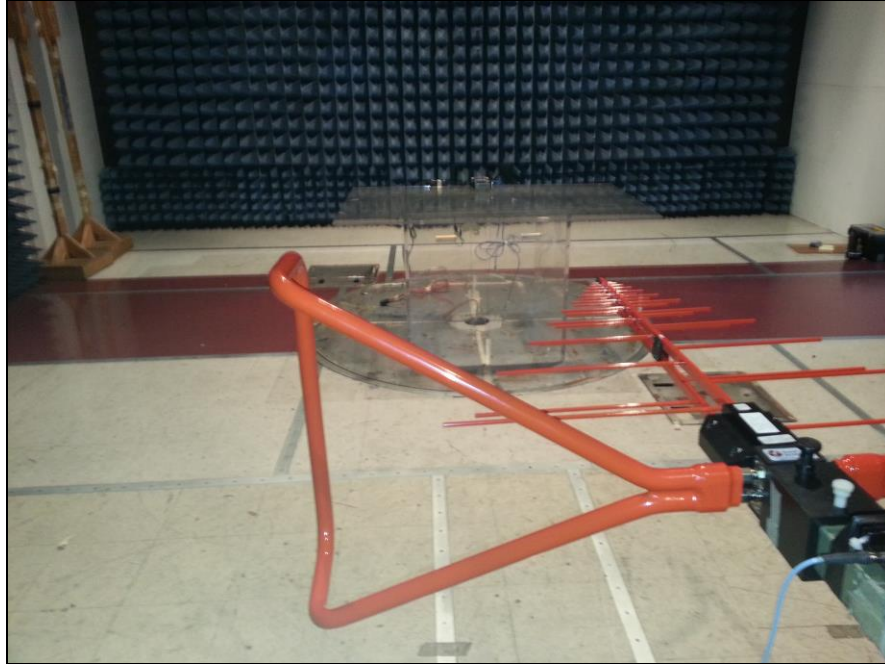
Photograph 3. Radiated Emissions, Test Setup, 30 MHz – 1 GHz
