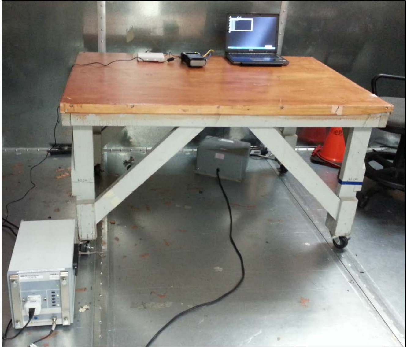
Photograph 2. Conducted Emissions, Test Setup
