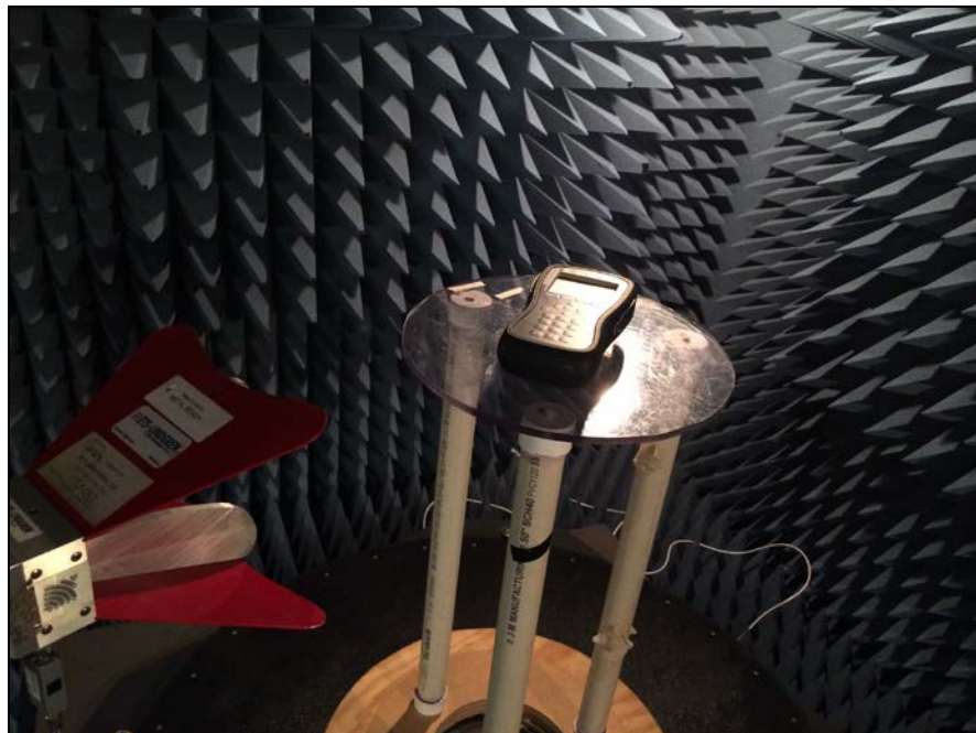
Photograph 7. Radiated Spurious Emissions, Test Setup Above 1 GHz
