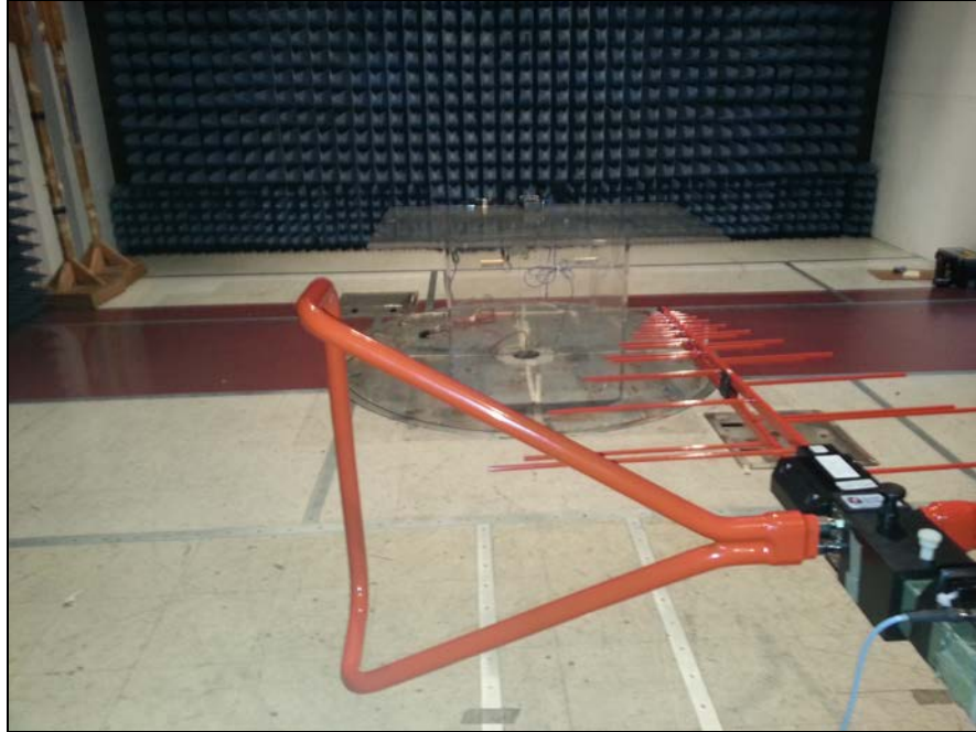
Photograph 3. Radiated Emissions, Test Setup, 30 MHz – 1 GHz
