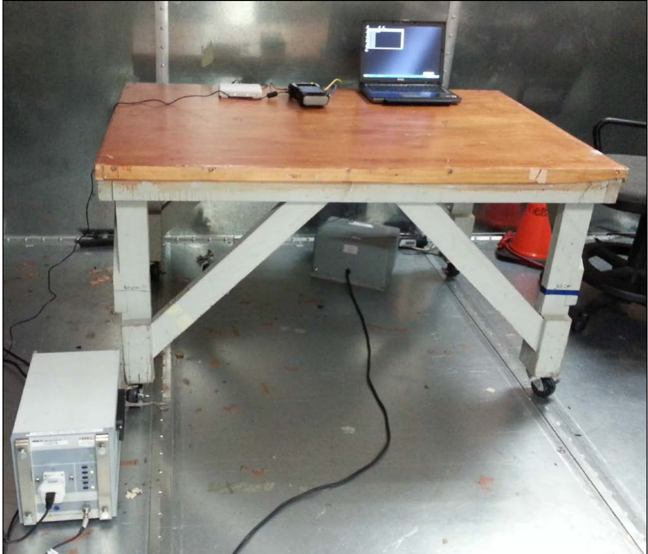
Photograph 5. Conducted Emissions, 15.207(a), Test Setup
