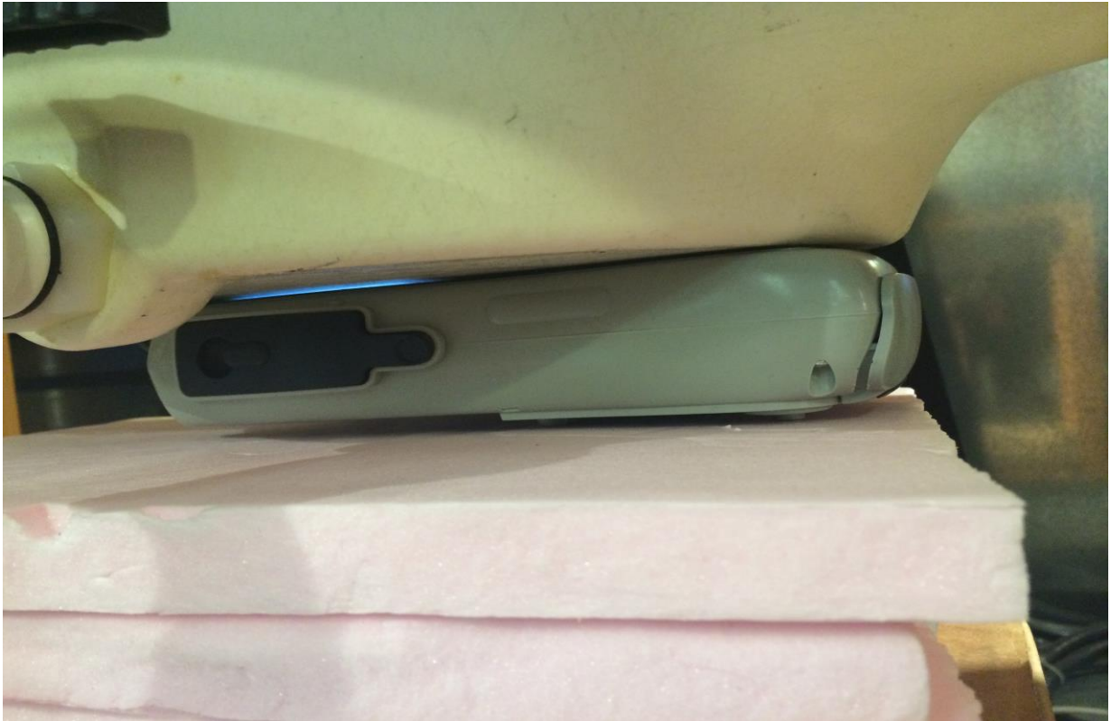
Photograph 2. EUT with Face of EUT against Phantom
