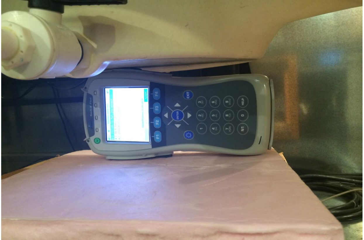
Photograph 1. EUT Right Edge/Antenna, Side against Phantom
