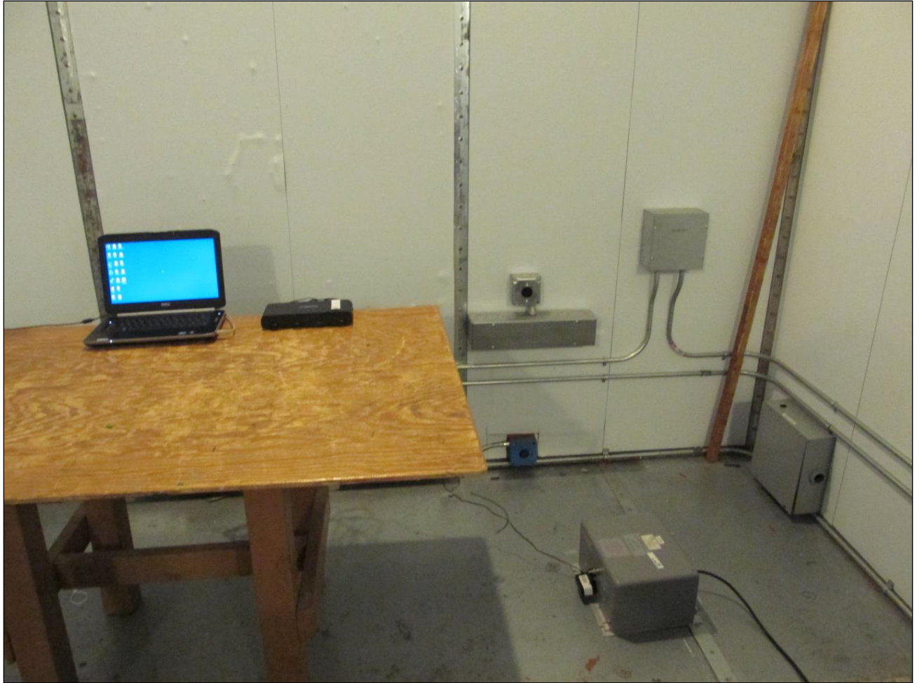
Photograph 3. Conducted Emissions, 15.207(a), Test Setup
