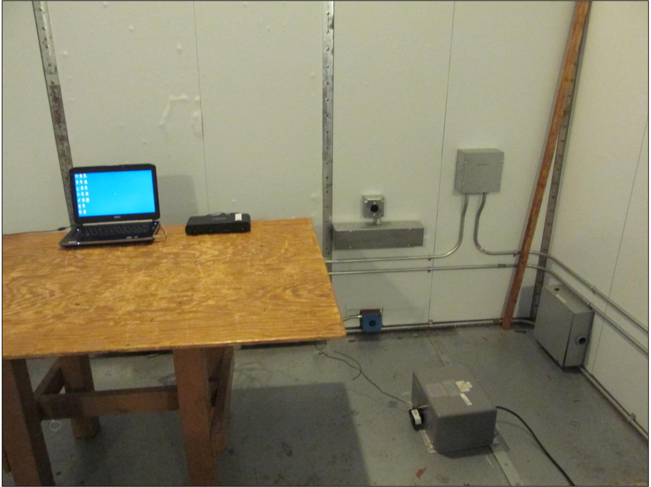
Photograph 1. Conducted Emissions, Test Setup
