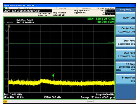
Test Plots (GFSK)- 5 GHz - 7 GHz Spurious Emission (CH.0)
