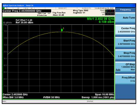
Test Plots (π/4DQPSK) Peak Power (CH.39)
