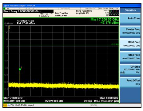
Test Plots(GFSK)- 9 GHz - 11 GHz Spurious Emission (CH.0)
