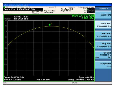
Test Plots (8DPSK) Peak Power (CH.0)
