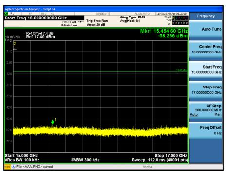
Test Plots(GFSK)- 17 GHz - 19 GHz Spurious Emission (CH.0)
