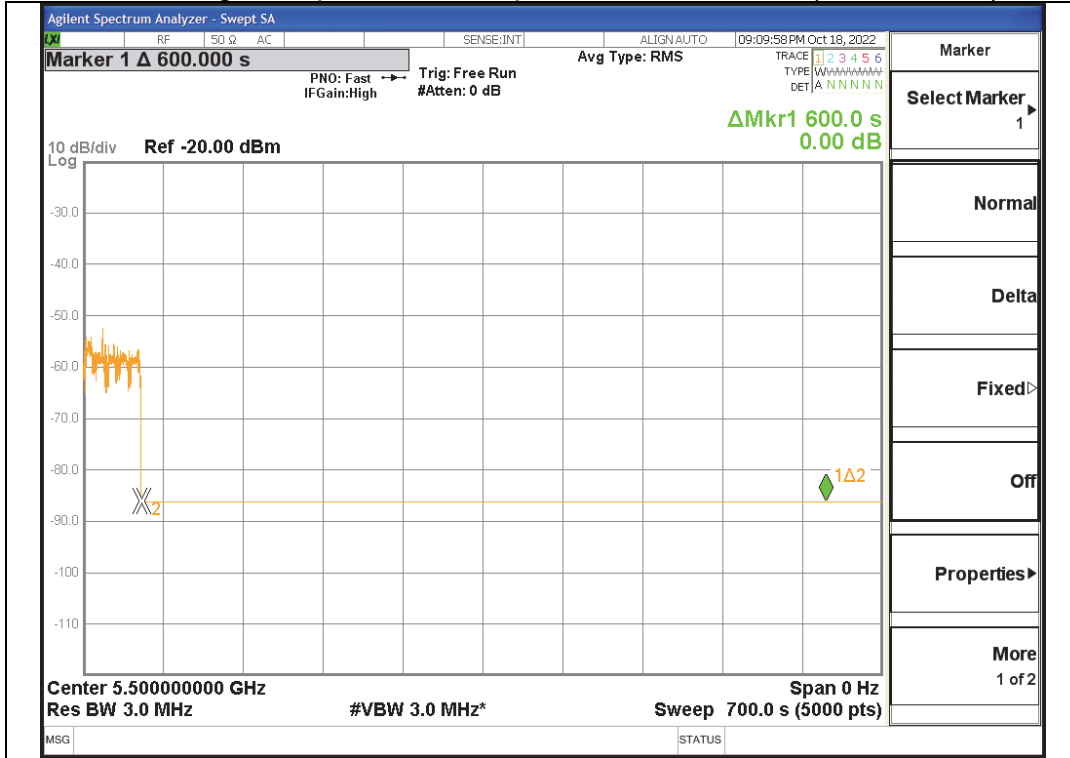
Monitoring live spectrum – Elapse time 30 minutes (20 MHz BW)
