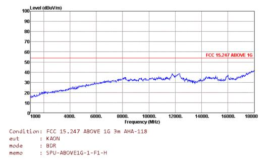
Note : 1) Only the worst case plots for Radiated Spurious Emissions. 2) A filter was used for this test.
