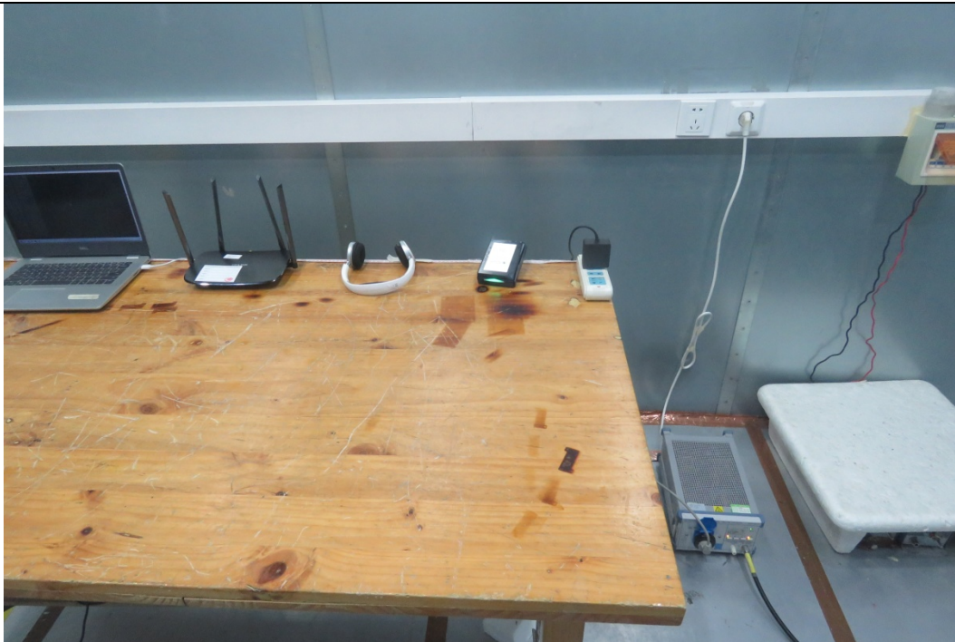
Picture 2: Conducted Emissions Test Setup
