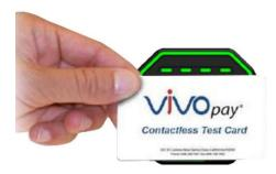
The antenna should beep, and the four green LEDs should illuminate in sequence, then all will illuminate together, briefly (750 msec), to indicate a successful test.
