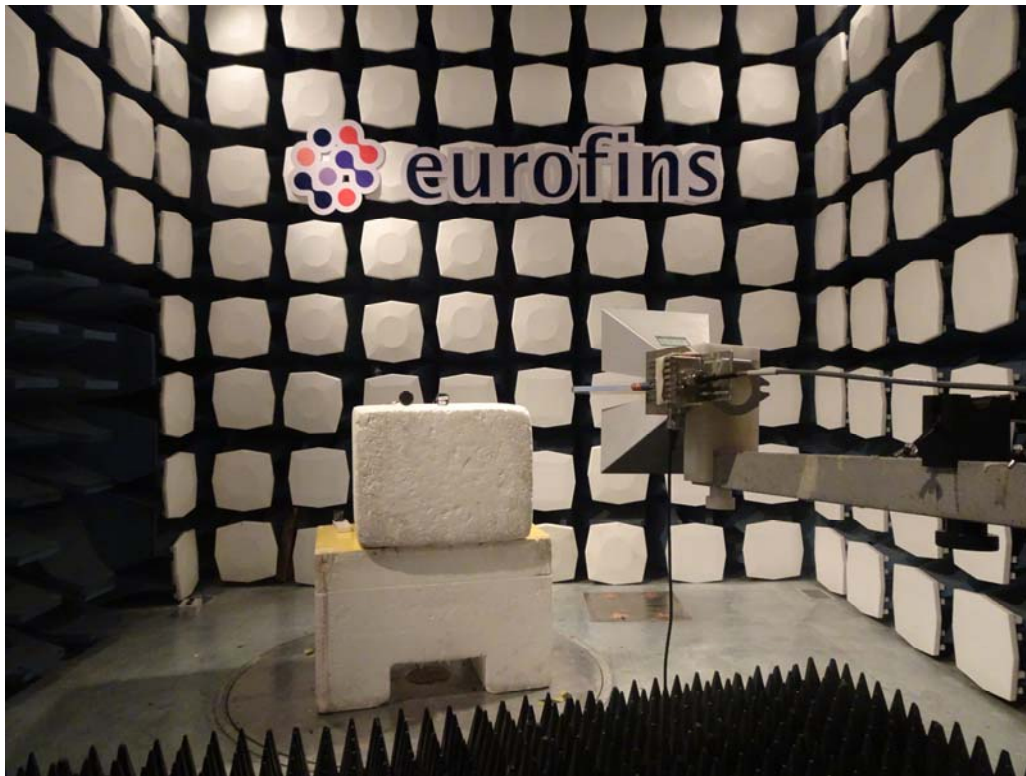
Picture 1: Radiated Spurious Emissions Test setup
