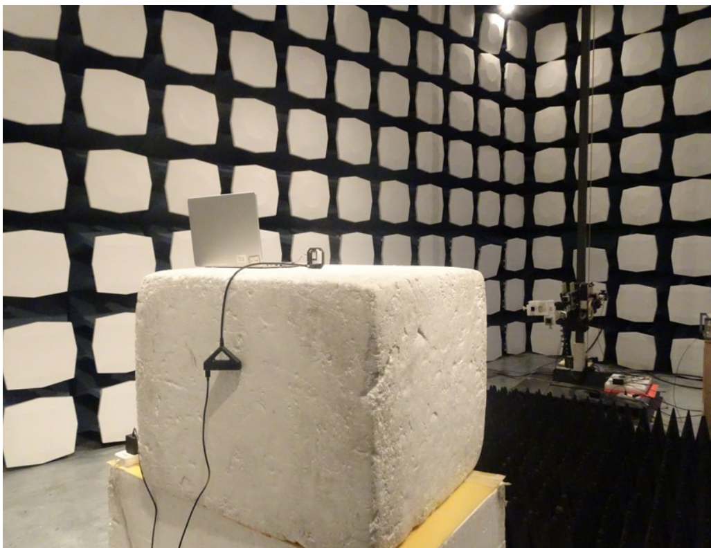
Picture 1 Radiated Emission Test Setup
