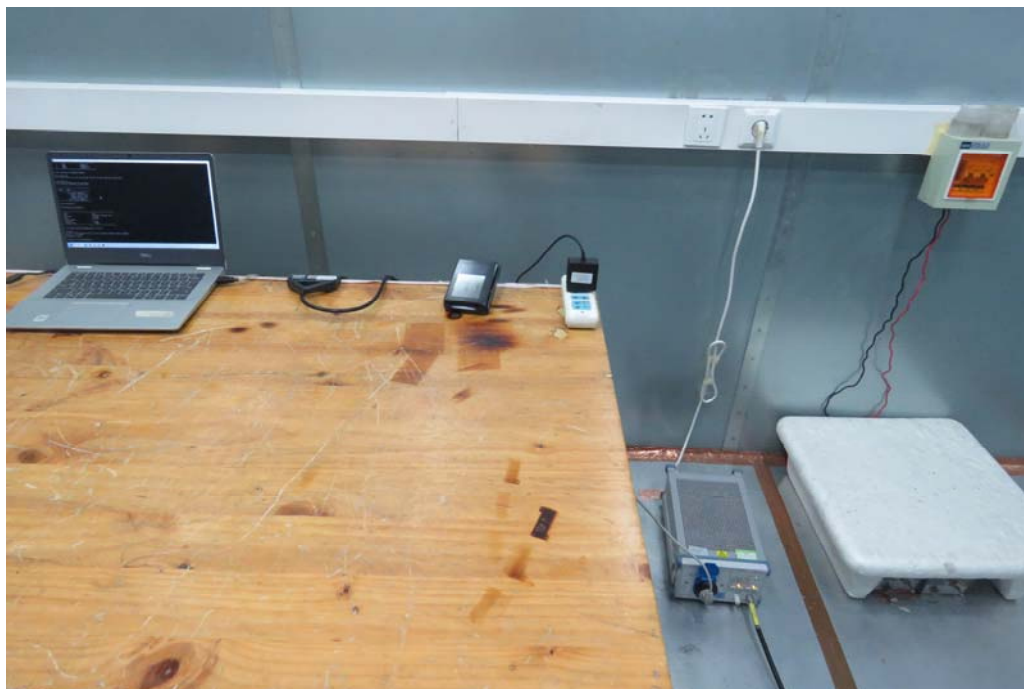
Picture 2 Conducted Emission Test Setup
