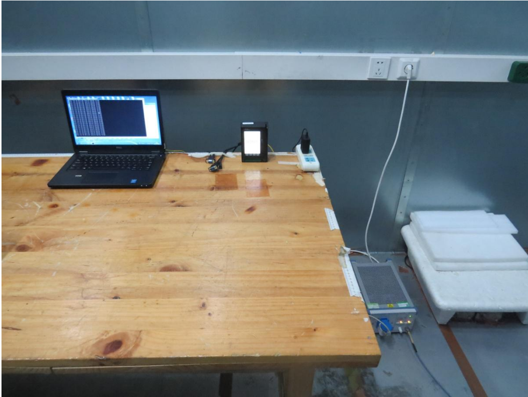
Picture 3 Conducted Emission Test Setup
