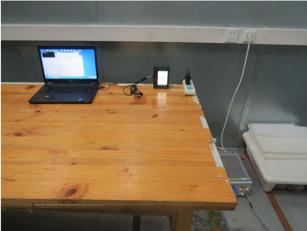
Picture 3 Conducted Emission Test Setup
