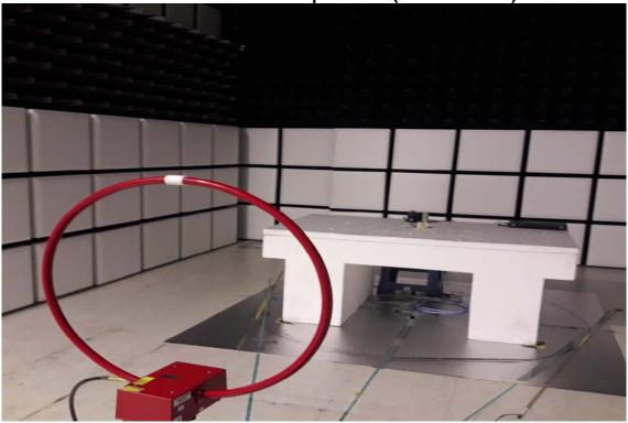
Radiated Emission Setup Photos (Below 1GHz)
