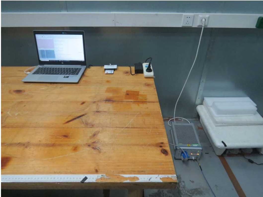
Picture 3 Conducted Emission Test Setup
