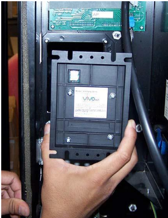
Figure 3. Placing the reader (ViVOpay Vend shown)
