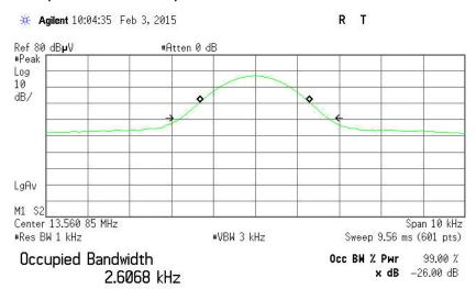
Transmit Freq Error -21.238 Hz x dB Bandwidth 3.507 kHz
