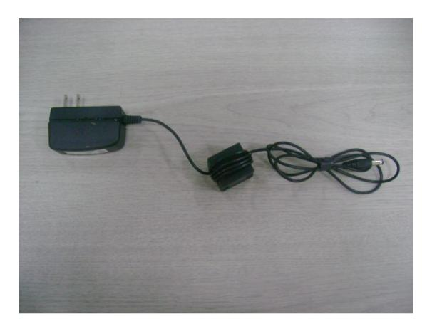
The coil has 4 circle power cable, the coil part number: HFB160093-300
