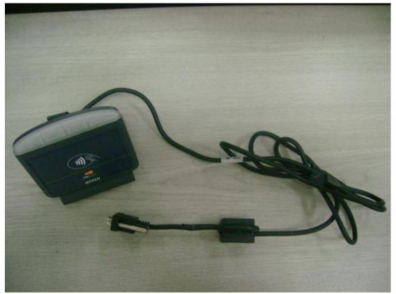
The Rs232 coil has one circle of Rs232 cable, the coil part number: HFB160093-300
