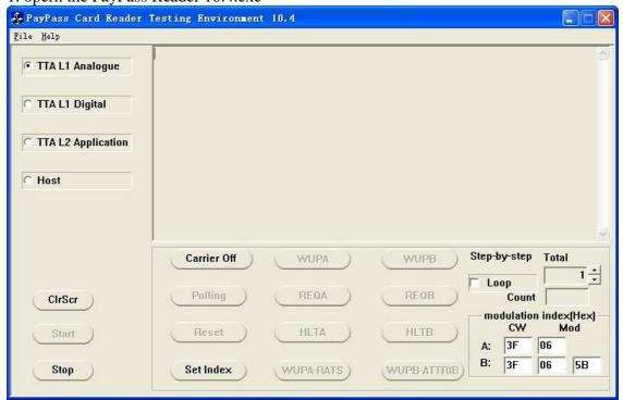
2.click the "Carrier ON",then the demo card can be tested. Put the card on Xpress reader.
