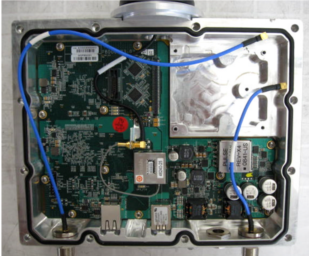
Photograph No.2 Base station WiN7237 internal view with RF module removed
