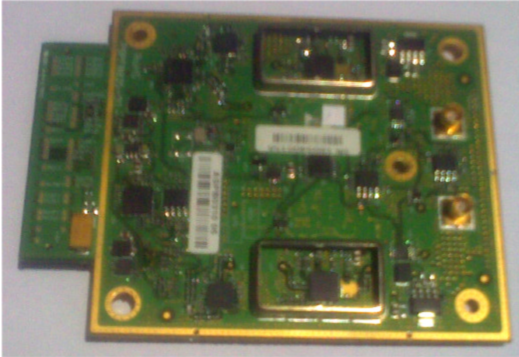
Photograph No.9 RF module front view without shields
