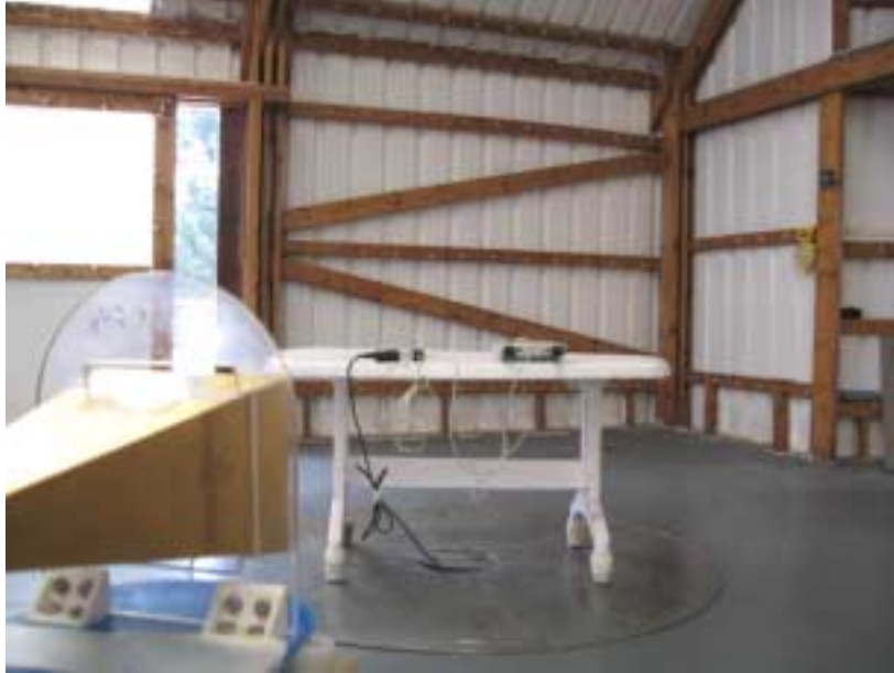
Photograph No.6 Radiated spurious emissions measurement setup at the OATS above 1000 M
