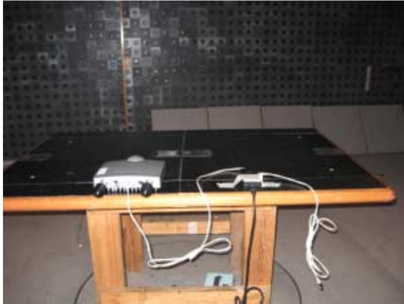
Photograph No.5 Spurious emissions measurement setup, EUT close view
