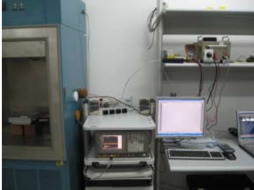
Photograph No.9 Frequency stability measurement setup
