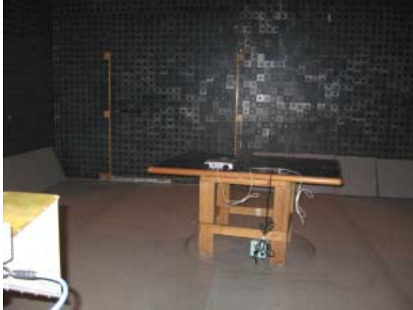
Photograph No.4 Spurious emissions measurement setup in the anechoic chamber above 1000 MHz
