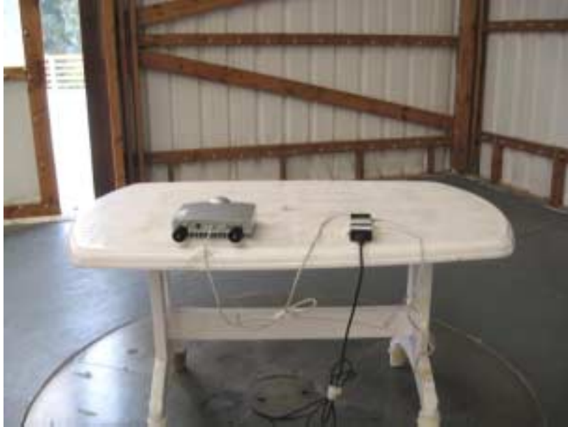
Photograph No.7 Radiated spurious emissions measurement setup at the OATS, close view
