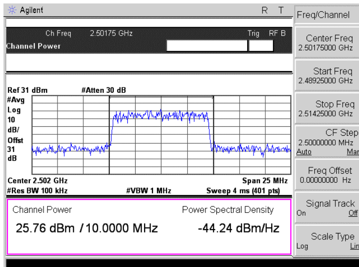
Plot 7.2.22 Peak output power test results at low frequency, 10 MHz, QPSK (Tx gain 11)
