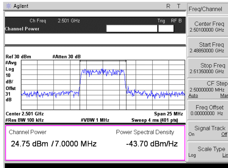
Plot 7.2.16 Peak output power test results at low frequency, 7 MHz, 16QAM (Tx gain 10)
