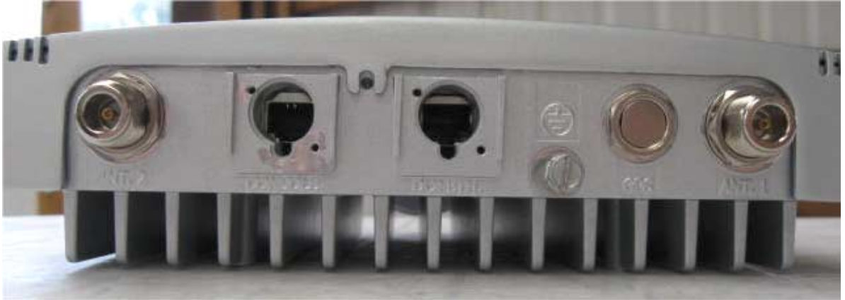
Photograph No.3 Base station WiN7225 RF connectors
