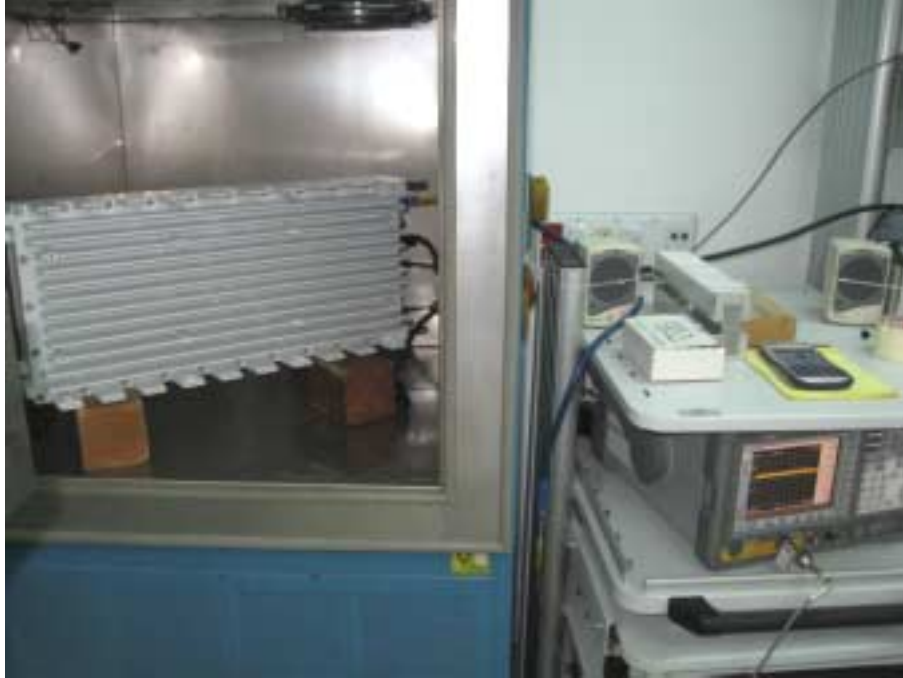
Photograph No.10 Frequency stability measurement setup
