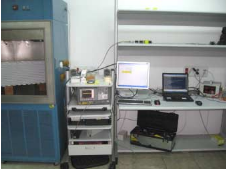
Photograph No.2 Conducted spurious emissions measurement setup
