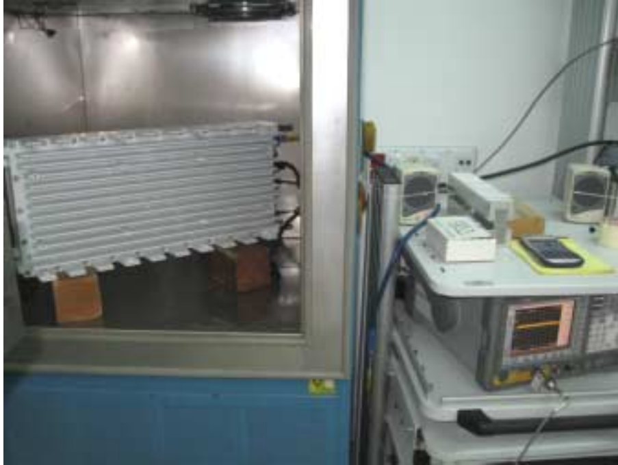
Photograph No.1 Peak output power, power spectral density, occupied bandwidth measurement setup
