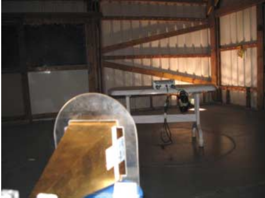
Photograph No.8 Radiated spurious emissions measurement setup at the OATS above 1000 MHz
