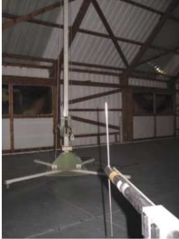
Photograph No.9 Substitution ERP measurements of spurious setup at the OATS
