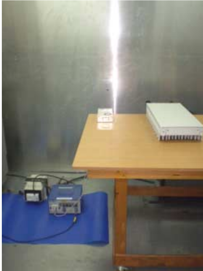
Photograph No.11 Conducted emissions measurement on AC line setup
