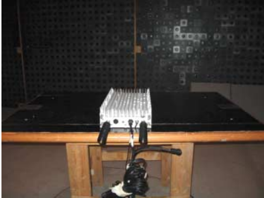
Photograph No.6 Spurious emissions measurement setup, EUT close view
