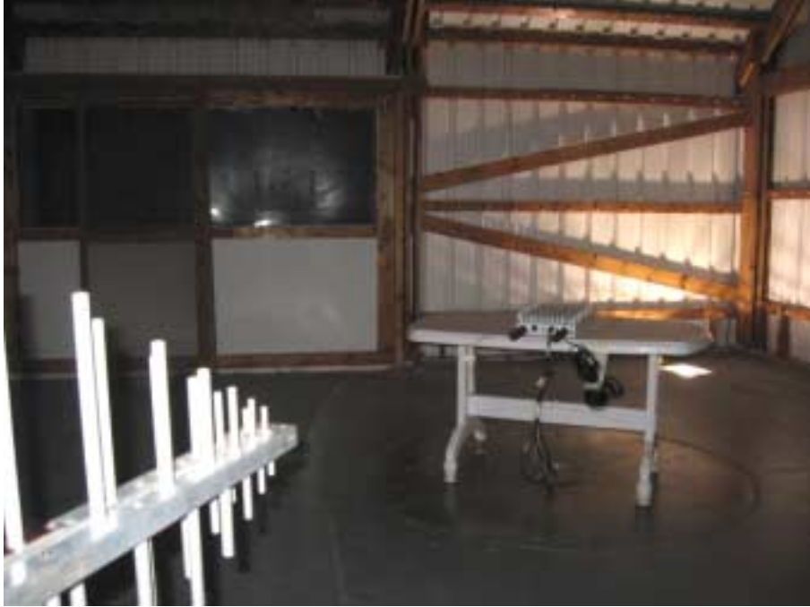
Photograph No.7 Radiated spurious emissions measurement setup at the OATS in 30 - 1000 MHz
