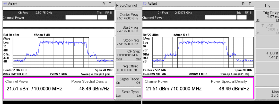
Plot 7.2.25 Peak output power test results at low frequency, 10 MHz, 16QAM
