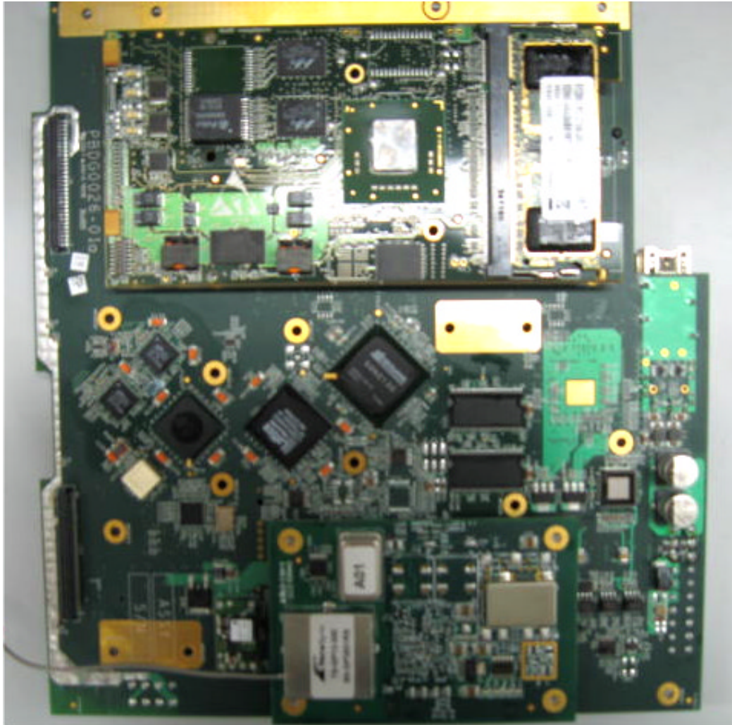
Photograph No.4 Main PCB second side view with GPS and CPU boards
