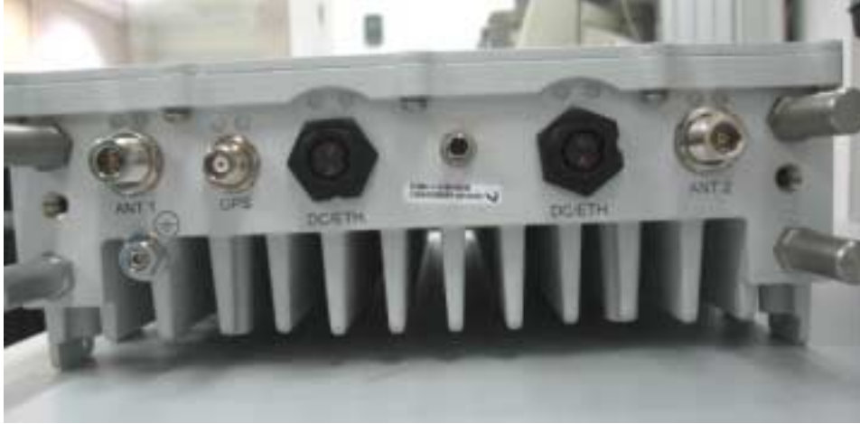
Photograph No.3 Base station WiN7025 RF connectors
