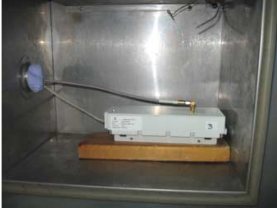
Photograph No.9 Frequency stability measurement setup
