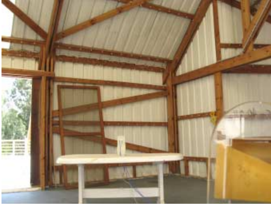
Photograph No.6 Radiated spurious emissions measurement setup at the OATS above 1000 MHz
