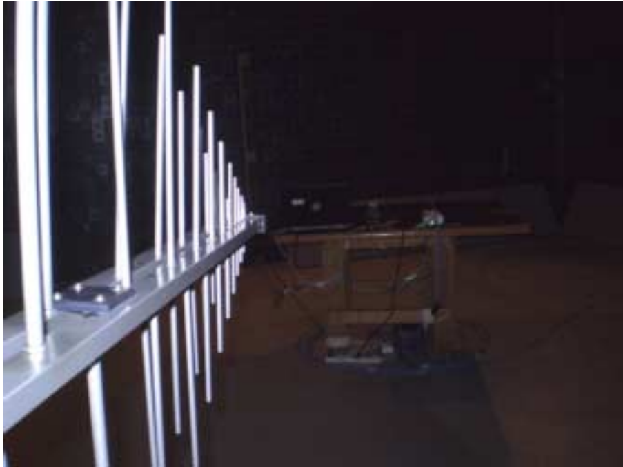
Photograph No.11 Radiated emissions measurement setup in the anechoic chamber in 30 -1000 MHz
