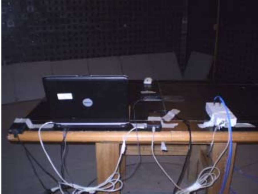
Photograph No.13 Radiated emissions measurement setup in the anechoic chamber, EUT close view
