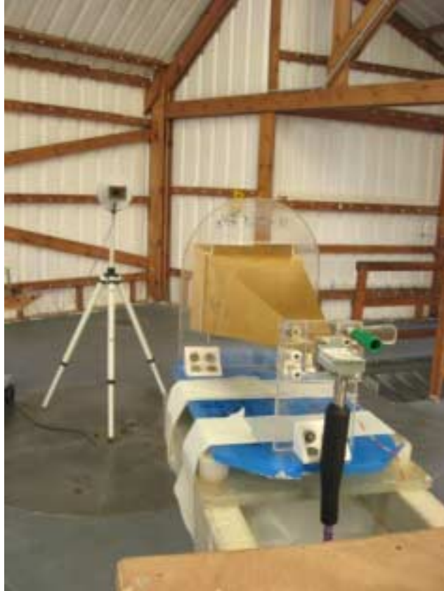
Photograph No.7 Substitution ERP measurements of spurious setup at the OATS
