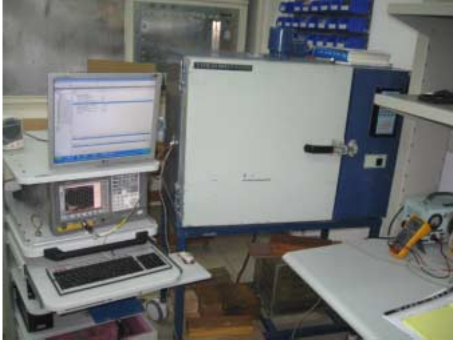
Photograph No.8 Frequency stability measurement setup
