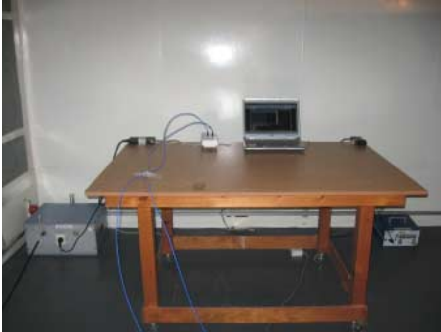
Photograph No.10 Conducted emissions measurement on AC line setup
