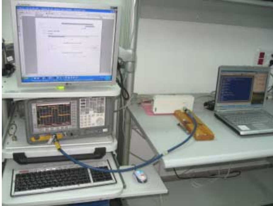
Photograph No.1 Peak output power, power spectral density, occupied bandwidth, emission mask, conducted spurious emissions measurement setup
