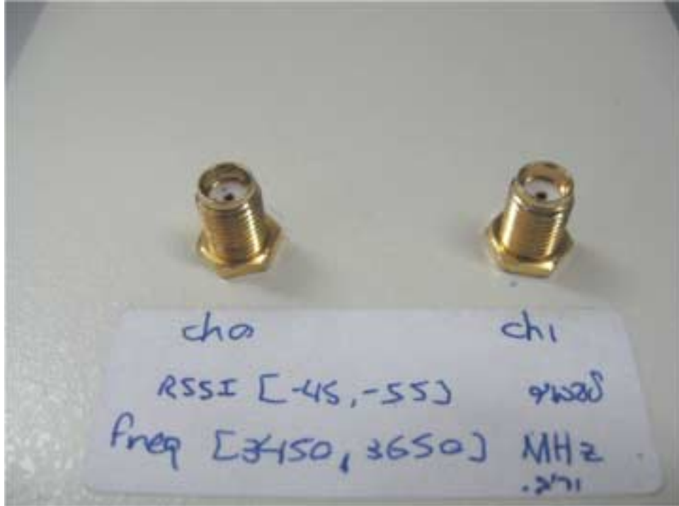
Photograph No.4 Subscriber unit WiN5235 RF connectors
