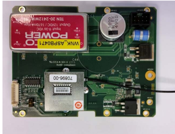
WIN5137-V-GPS PSU board – Front view
