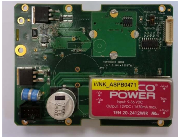
WIN5137-V PSU board – Front view
