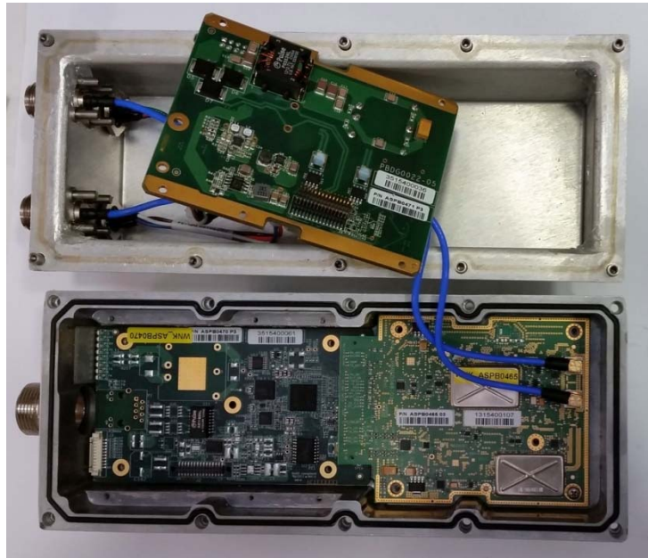
WIN5137-V Internal view – Without PSU board
