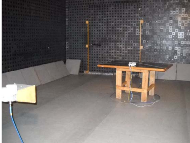
Photograph No.5 Spurious emissions measurement setup in the anechoic chamber in 1 - 18 GHz
