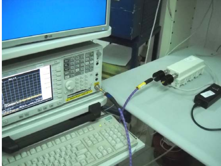
Photograph No.2 Conducted spurious emissions measurement setup
