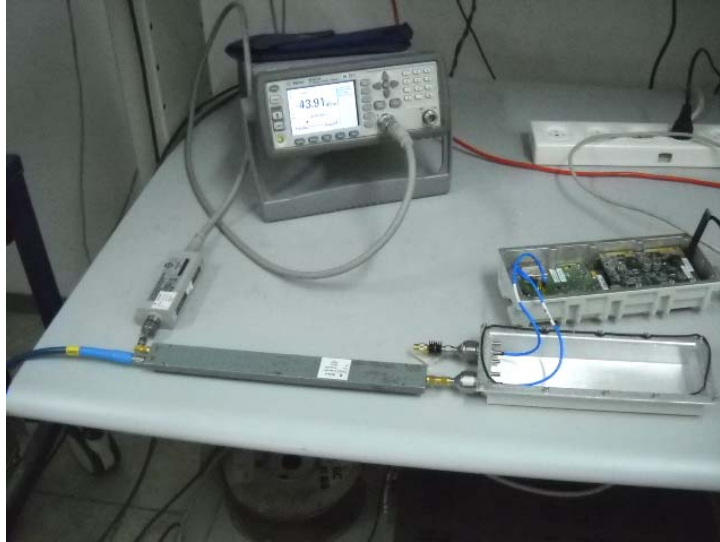
Photograph No.1 Peak output power, power spectral density, occupied bandwidth, emission mask measurement setup
