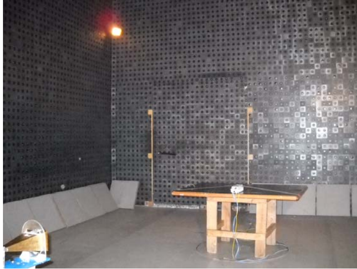
Photograph No.6 Spurious emissions measurement setup in the anechoic chamber above 18 GHz
