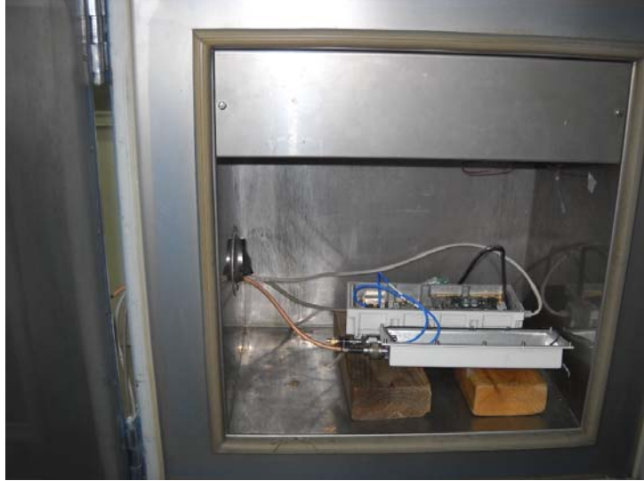
Photograph No.7 Frequency stability measurement setup
